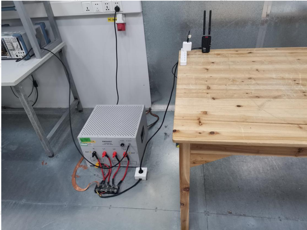
Photo of Power Line Conducted Emission Test
