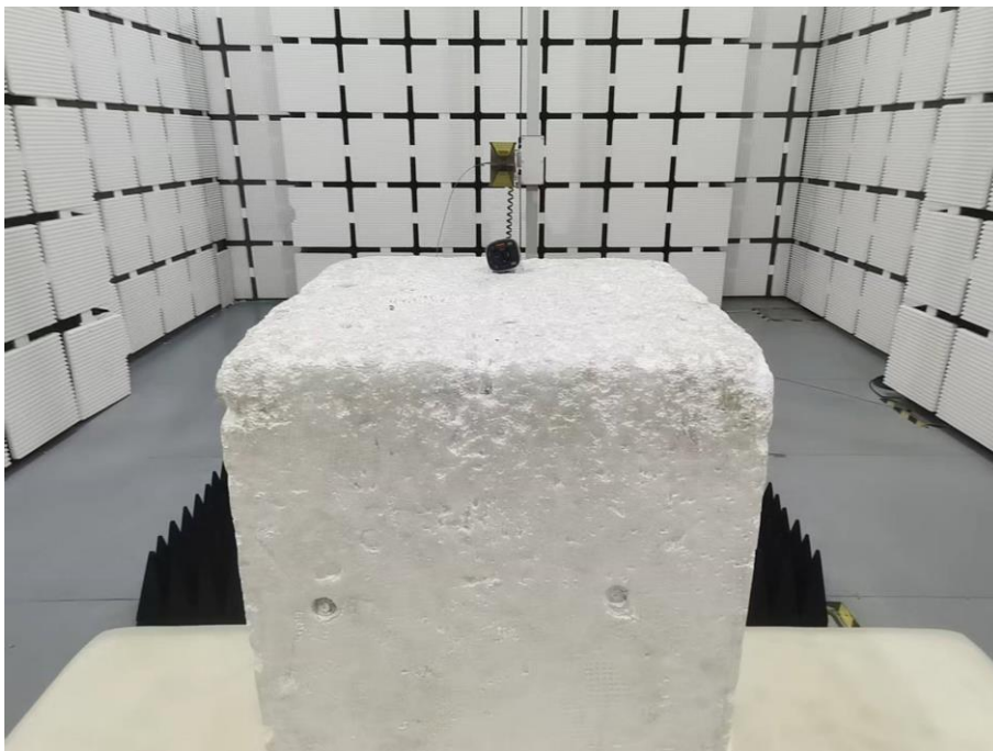
Set-up for Radiated Spurious Emission, Above 1GHz
