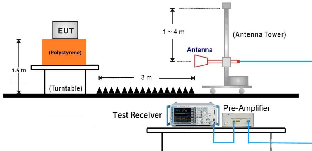
18GHz ~40GHz Test Setup:
