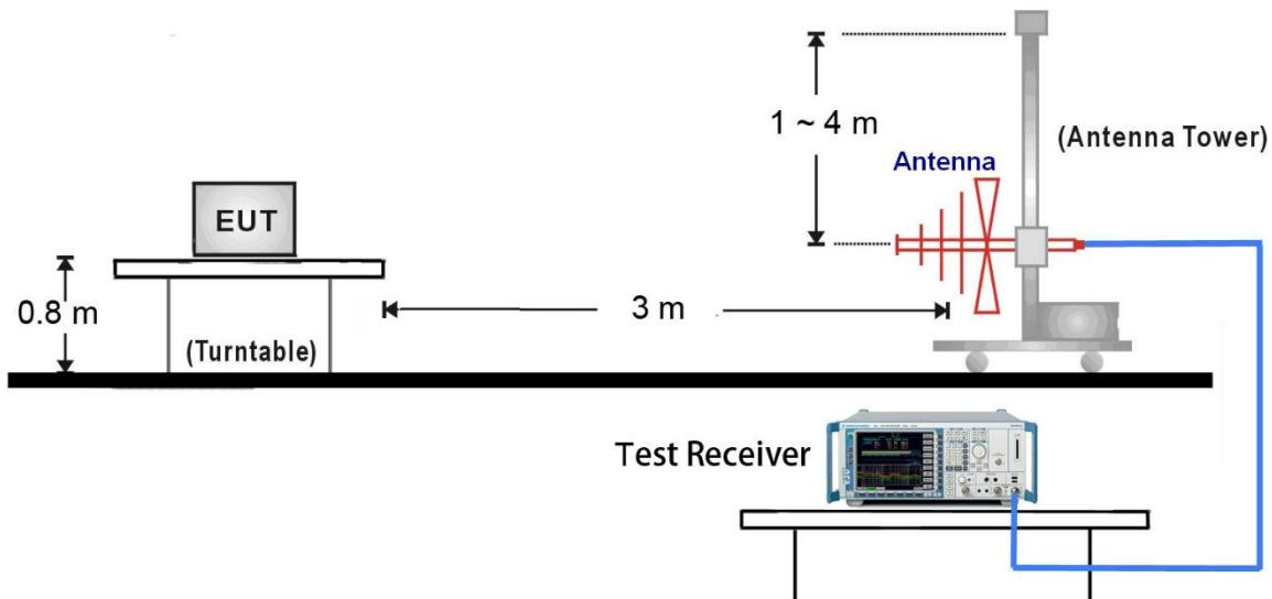
1GHz ~ 18GHz Test Setup:
