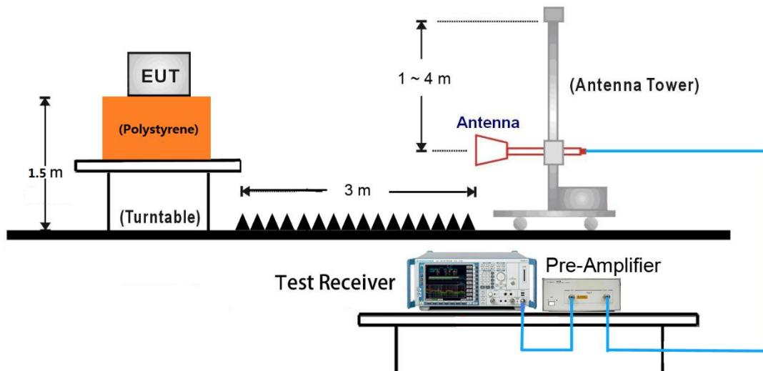
18GHz ~25GHz Test Setup:
