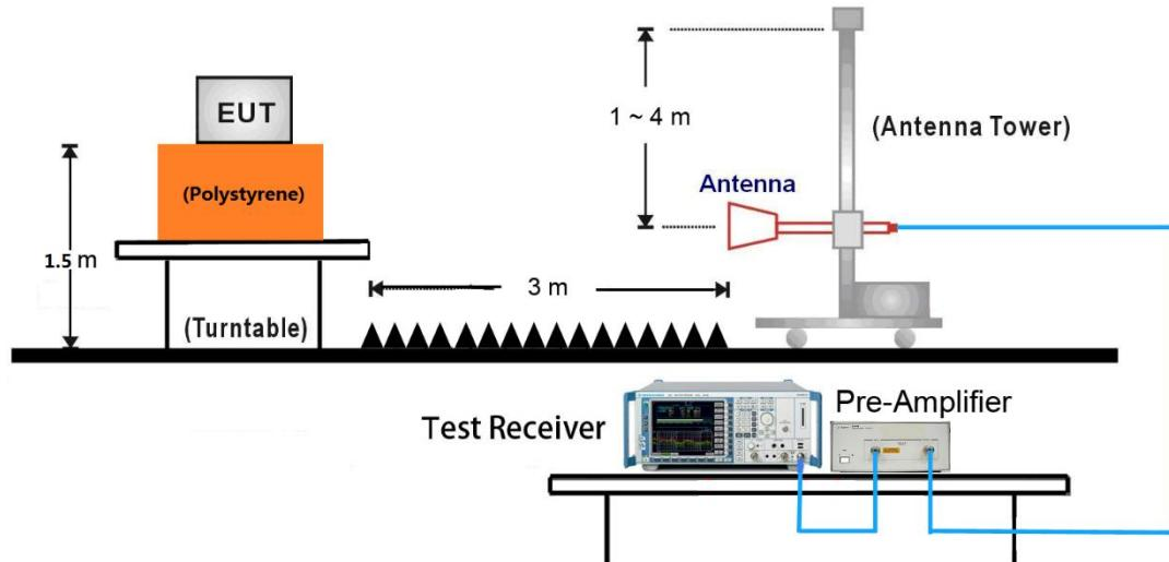
18GHz ~40GHz Test Setup:
