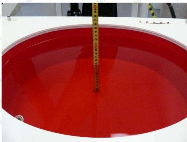
Liquid depth in Body Phantom (450MHz)
