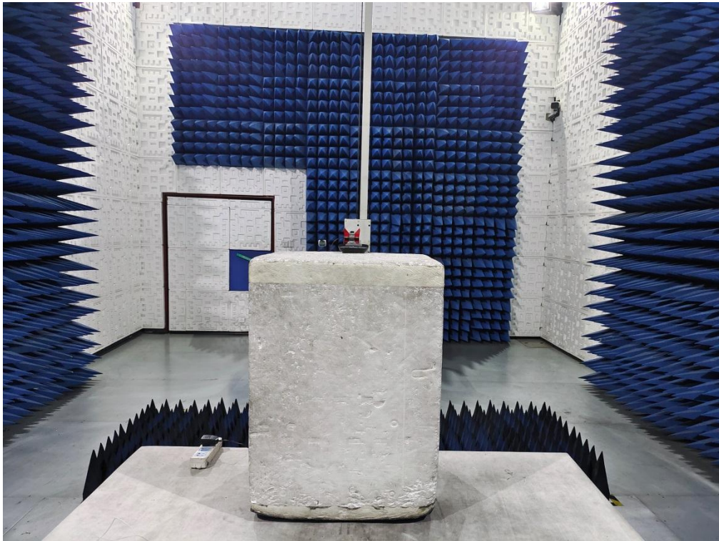
RADIATED EMISSION TEST SETUP ABOVE 1GHz
