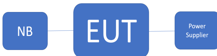
Fig. 2-1 Conducted (Antenna Port) & Radiated Emission Configuration & Emission from AC power line
