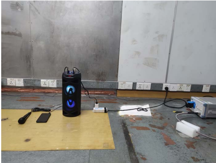
Photo of Power Line Conducted Emission Measurement
