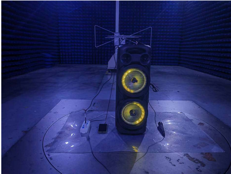
Photo of Radiated Emission Measurement Below 1GHz
