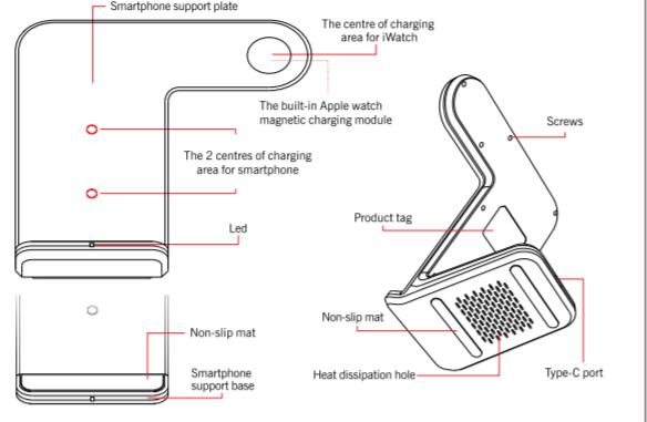
**Smartphone and iWatch Charging Schematic Diagram**
