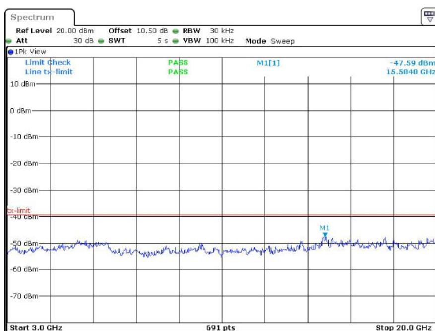
**Middle Channel (Unwanted Emission outside the Sub-band)**
