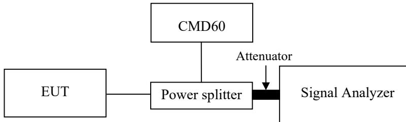
The width, in Hz, of the signal between two points, one below the carrier center frequency and one above the carrier center frequency, that is 26 dB down relative to the maximum level of the modulated carrier. It is based on the use of measurement instrumentation employing a peak detector function with an instrument resolution bandwidth approximately equal to 1% of the emission band-width of the device under measurement. [Extraction from 47 CFR 15, subpart D, 15.303 (C)].
