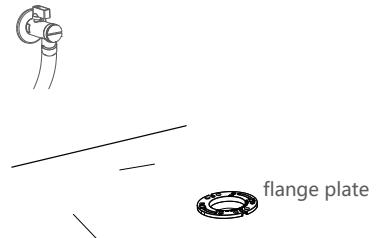
3. Place the bolt into the flange notch.
