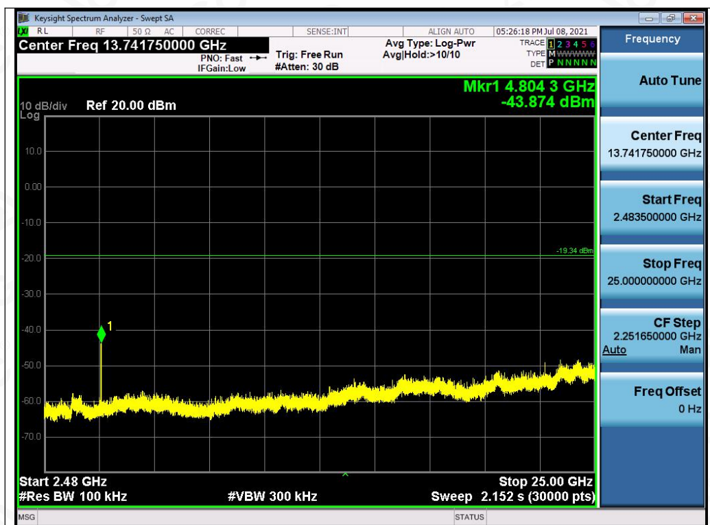
Test_Graph_BR_ANT1_2402_1Mbps_Higher Band Emissions
