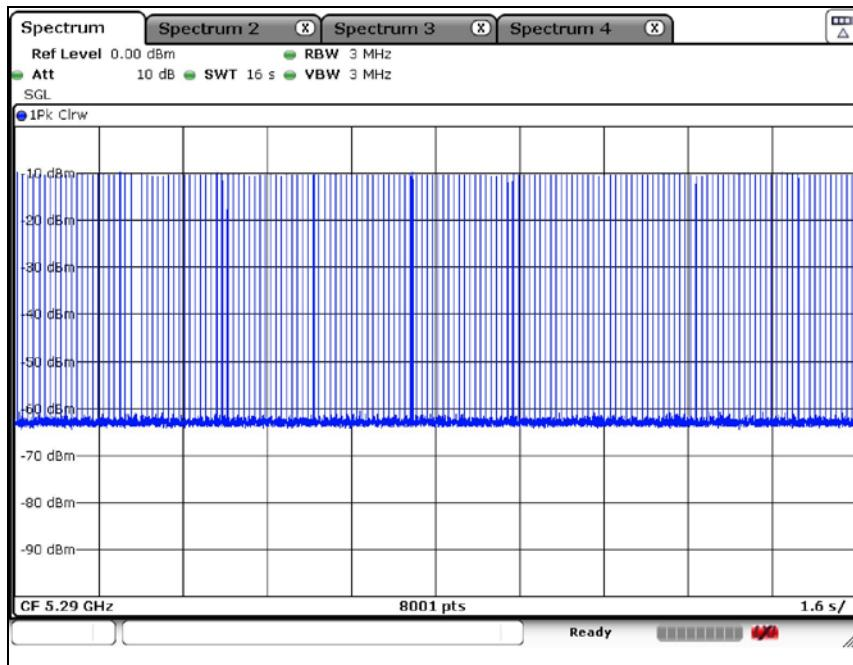
**11ac\_VHT80****5 530 MHz****Plot of LAN traffic**
