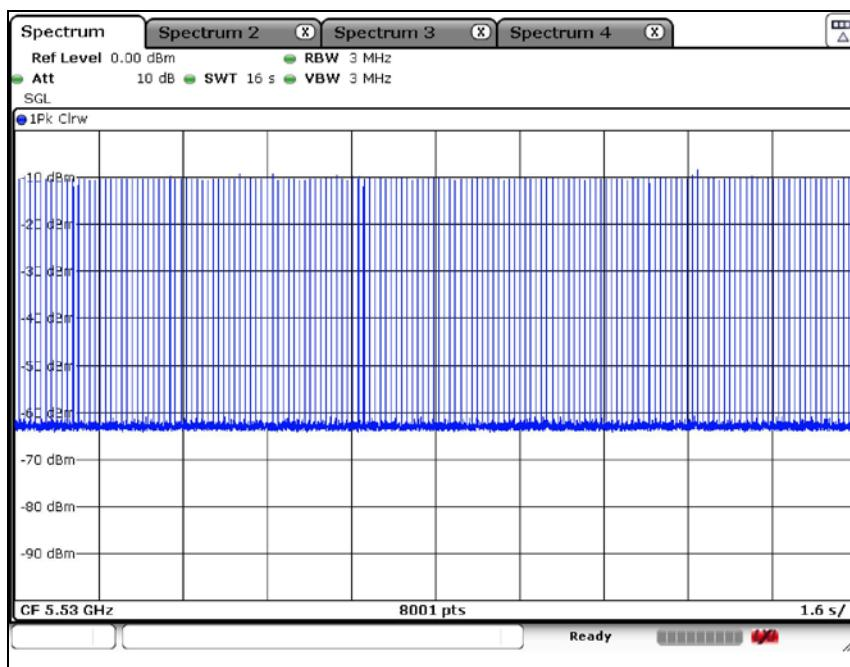
**Channel Loading****11ac\_VHT80****5 290 MHz**
