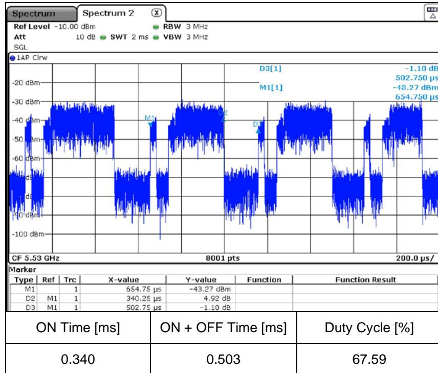
The reference maker is set after 200 ms from the end of Last radar pulse.
