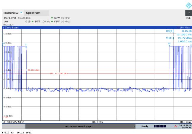
Duty cycle: Ton=8.582ms + 6.398ms = 14.98 ms. Ton+Toff=100ms
