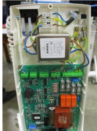
XRCC board assembled on cover
