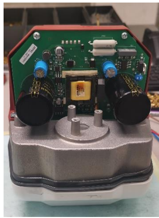
XRPS and XRHVP boards assembled
