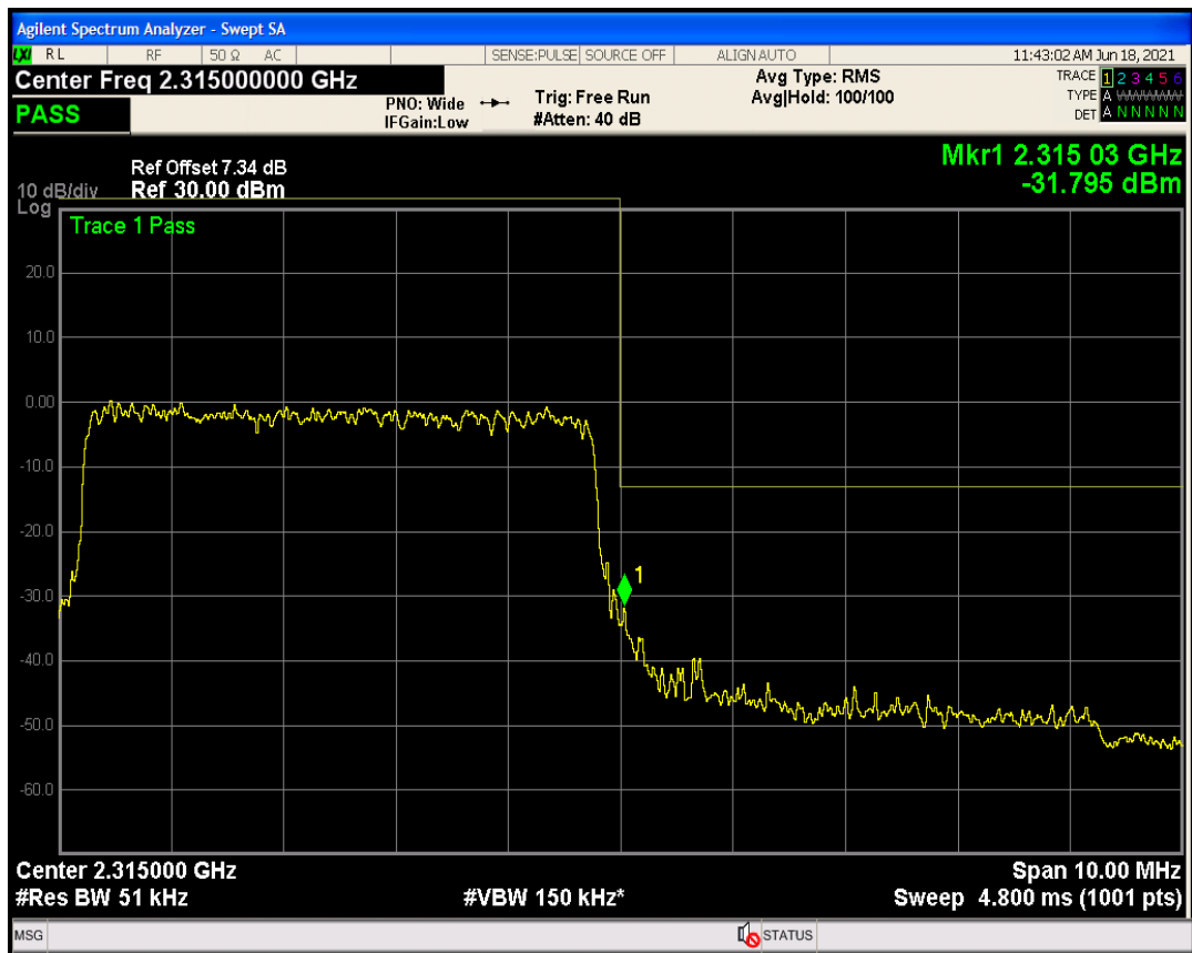
Band40a QAM16 BW=5MHz Channel=38775 RB Size=25 Position=#0
