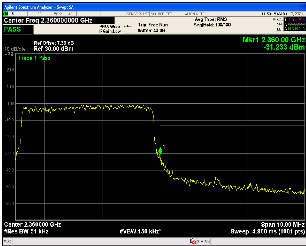
Band40b QPSK BW=10MHz Channel=39200 RB Size=50 Position=#0
