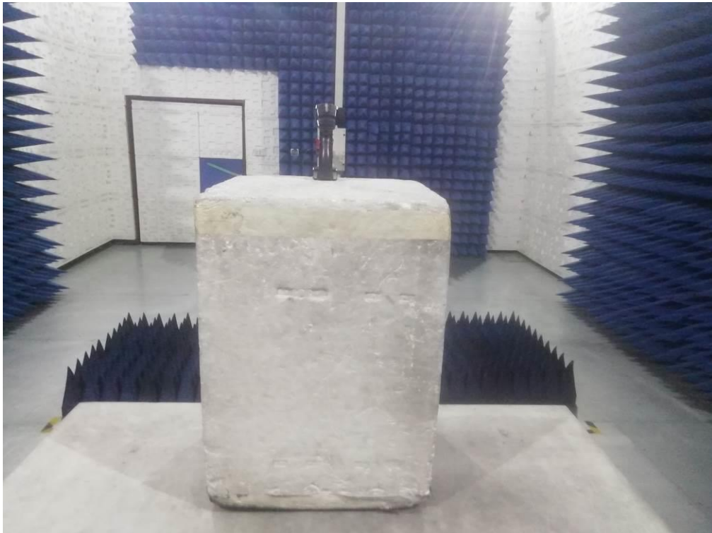
FCC RADIATED EMISSION TEST SETUP ABOVE 1GHZ
