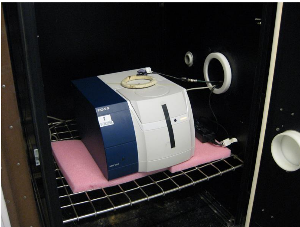
Photo 4.8.1 Test setup regarding measurement of Frequency stability.
