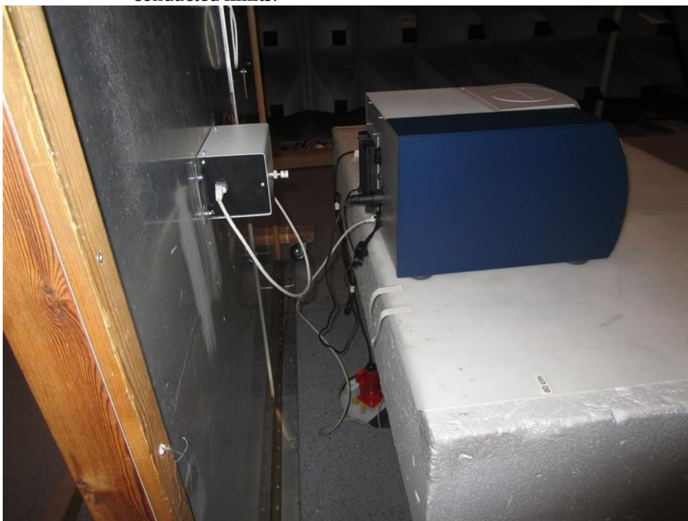
Photo 4.1.2 Test setup regarding measurement of radio frequency voltage on mains/ conducted limits.
