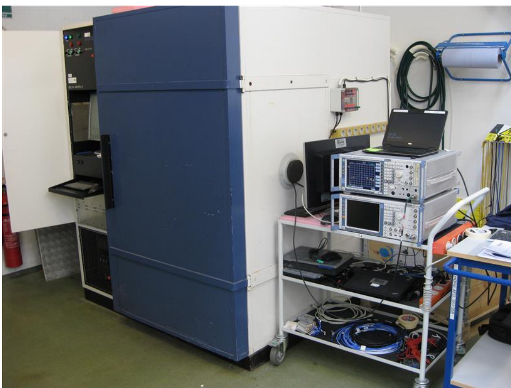
Photo 4.8.2 Test setup regarding measurement of Frequency stability.
