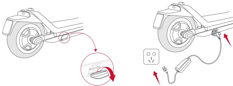
Firstly open the charging port, then plug the charging plug into the body charging port and finally connect the power supply to charge. After the completion of charging, fastening down the charging port to beware of water intake.
