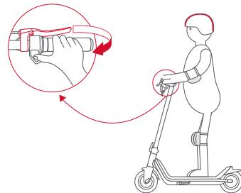
**04** Release the throttle twistgrip and use the energy recovery to achieve the effect of deceleration. Emergency braking requires powerful grip on both sides of the brake levers.
