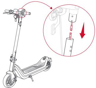
**04** Lock the screws on both sides alternately with the hexagon wrench in the packaging box (tightening torque: 4-5N\*m), that is, the assembly is completed.
