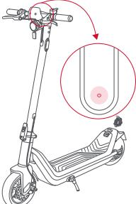
**02** Connect the handlebar to the main line connector of the vertical tube, and install the handlebar to the vertical tube .
