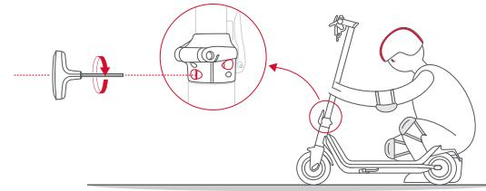
Check whether the vertical tube screws are loose. If so, fasten the standpipe screws first, and then fasten the two screws of the folding mechanism with a 6mm hexagon wrench.
