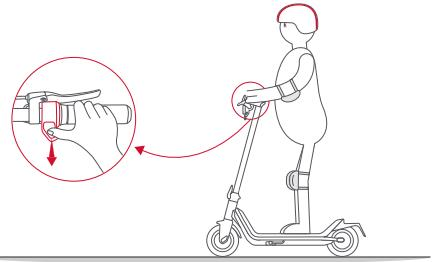
**03** When the kick scooter is sliding, stand on the pedal with the other foot, keep both feet stable, while gently pressing the throttle twistgrip. (The speed above 4km/h will start the throttle)
