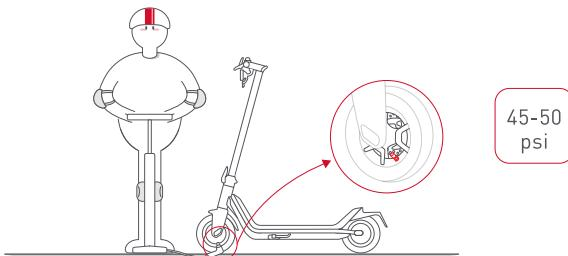
If your kick scooter front and rear tires are underinflated, please use the extension nozzle to connect the car body tires to inflate. First remove the front and rear tire inflatable nozzle cap, and then tighten the extended inflatable nozzle and tire inflatable nozzle, and connect the pump to inflate after they are to be tightened.
