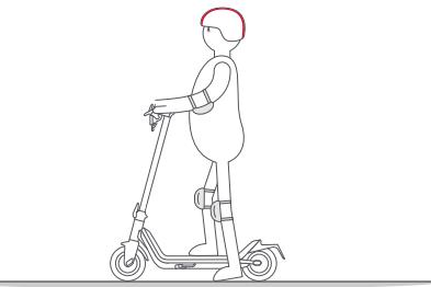
**02** Stand on the pedal with one foot and push back with the other foot.
