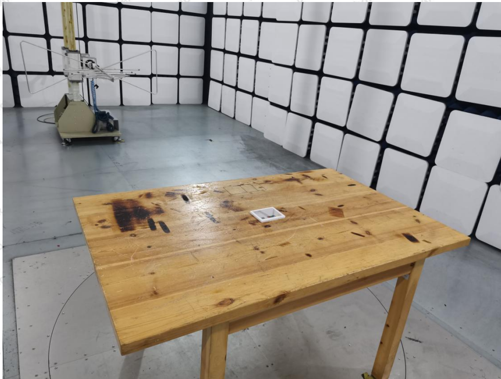
Photo of Radiation Emission Test
