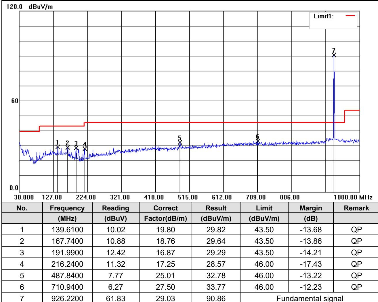
Level = Read Level + Antenna Factor + Cable Loss – Preamp Factor.
