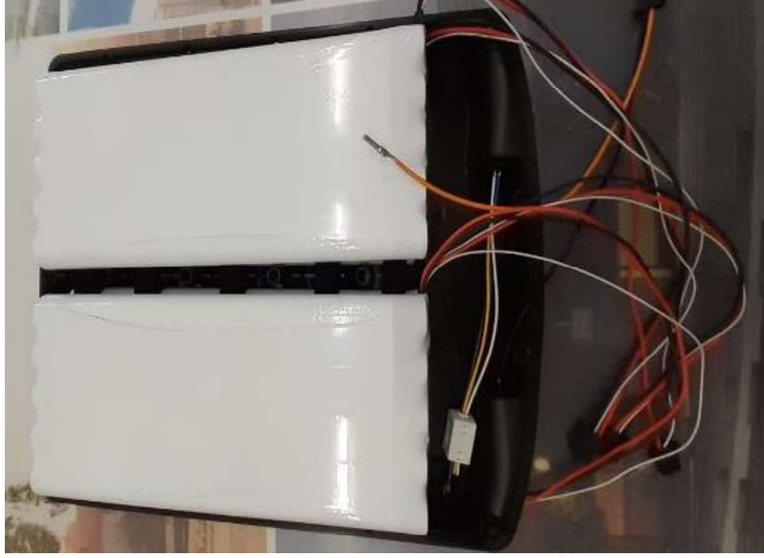
POWER 365 with 4 battery packs with the connections
