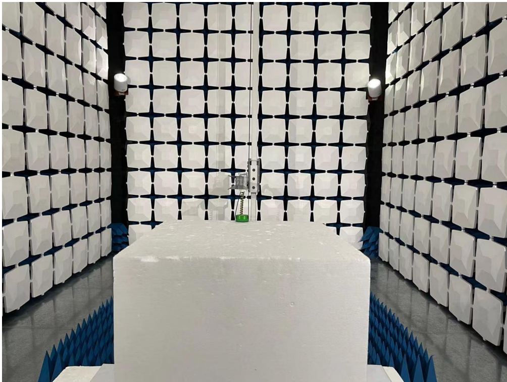
Above 1GHz for radiated emission test setup
