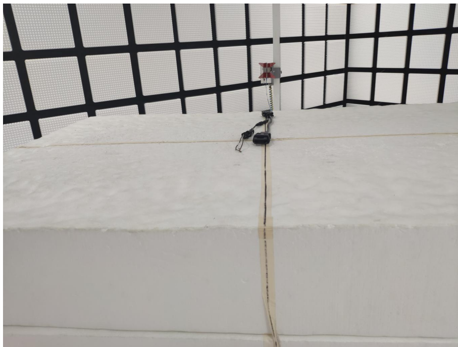
Radiated spurious emission Test Setup-3(Above 1GHz)
