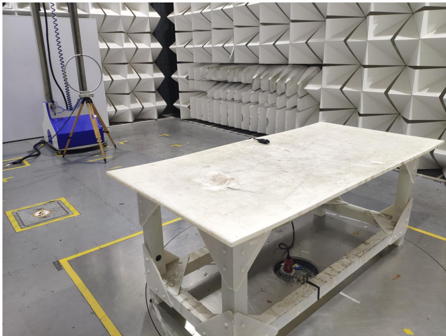
Radiated spurious emission Test Setup-1(Below 30MHz)
