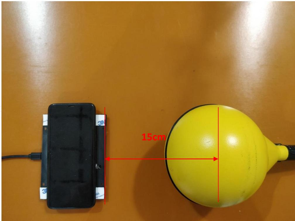
**9.4. Test Position D - Exposure photo from side edge surface-Right**
