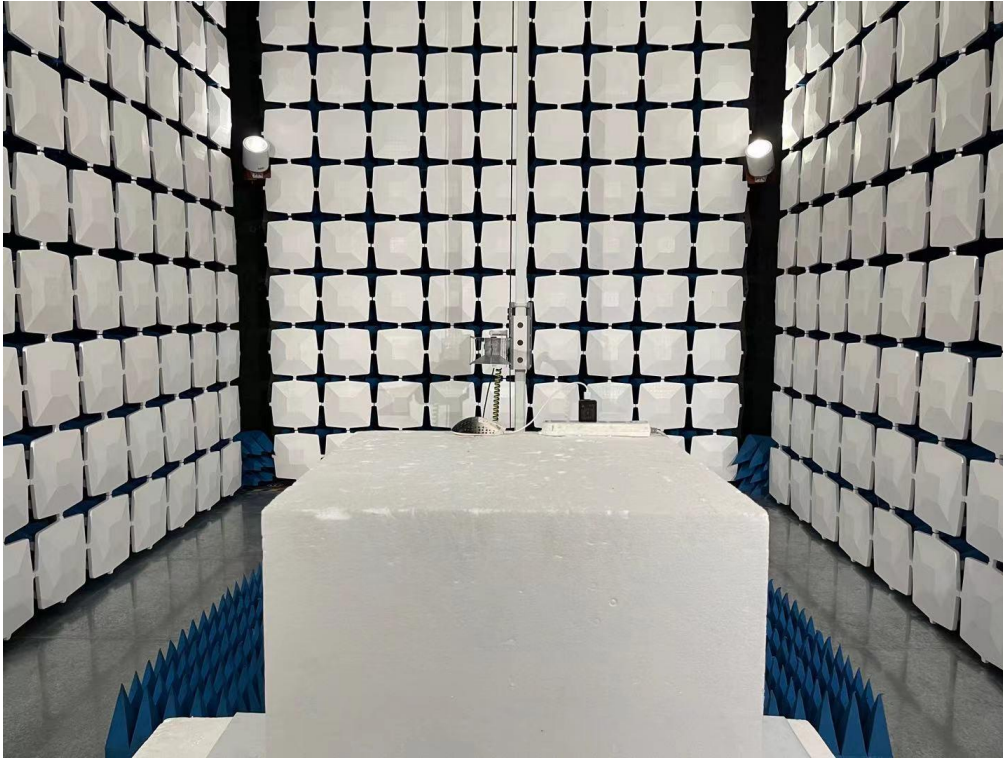
Above 1GHz for radiated emission test setup
