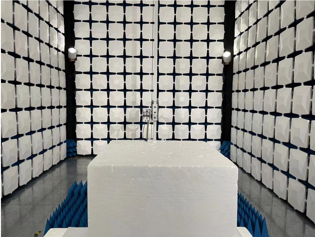
Above 1GHz for radiated emission test setup
