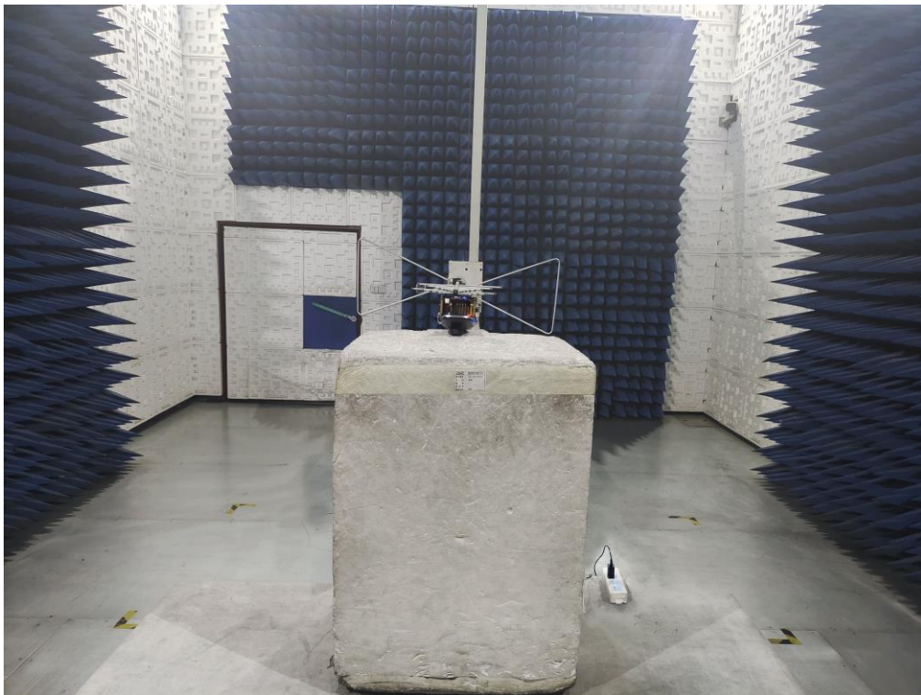
FCC RADIATED EMISSION TEST SETUP 30MHz-1GHZ
