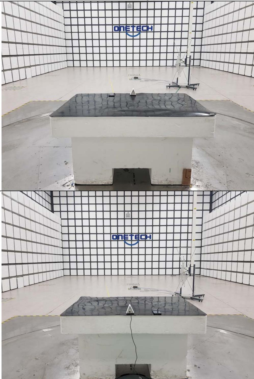
**Radiated Disturbance Test Set Up (Above 1 GHz)**
