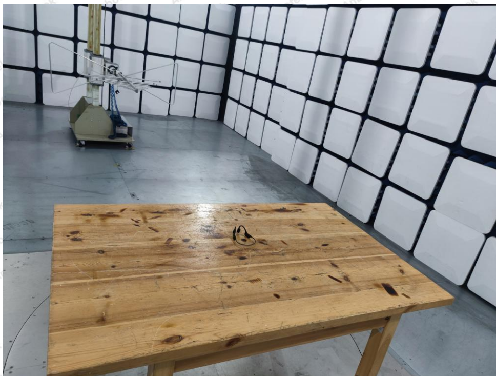
Photo of Radiation Emission Test
