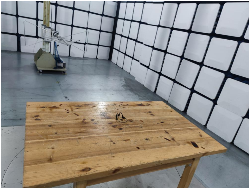
Photo of Radiation Emission Test
