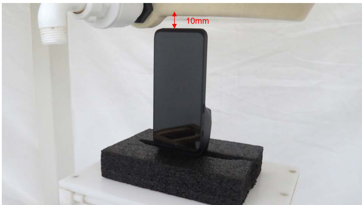
Picture 8: Bottom Edge, the distance from handset to the bottom of the Phantom is 10mm
