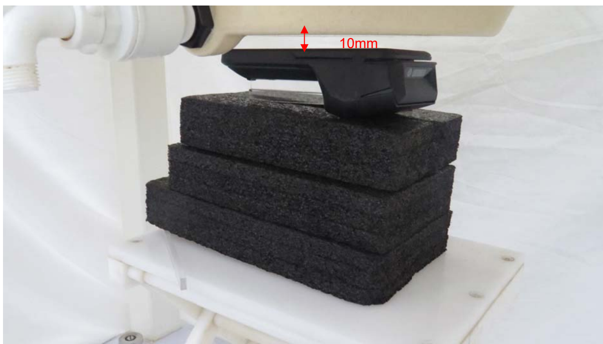
Picture 4: Front Side, the distance from handset to the bottom of the Phantom is 10mm
