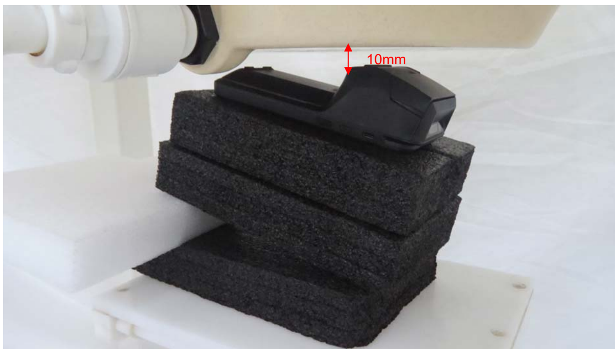
Picture 3: Back Side, the distance from handset to the bottom of the Phantom is 10mm
