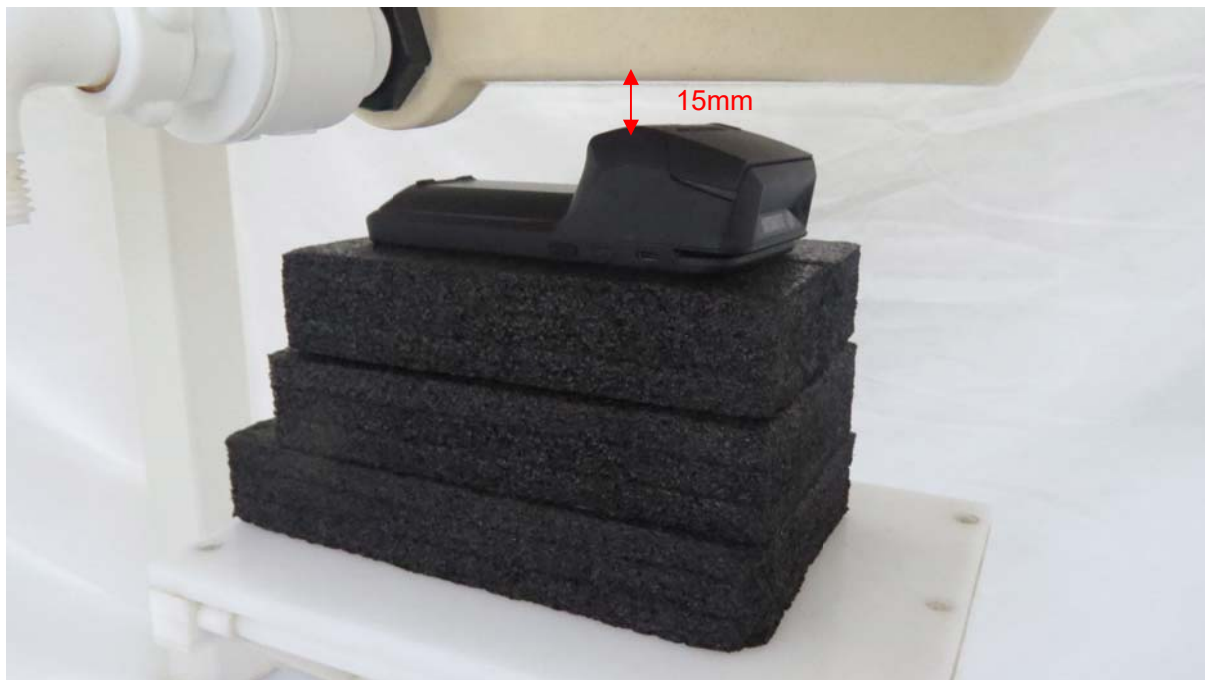
Picture 1: Back Side, the distance from handset to the bottom of the Phantom is 15mm
