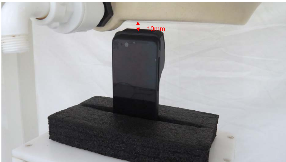
Picture 7: Top Edge, the distance from handset to the bottom of the Phantom is 10mm
