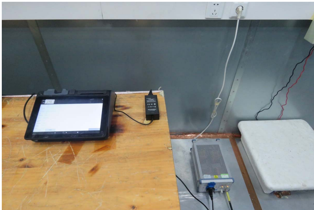
Picture 2 Conducted Emission Test Setup
