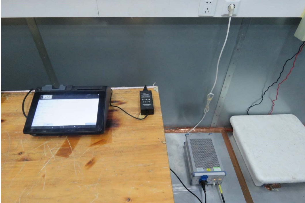
Picture 2 Conducted Emission Test Setup
