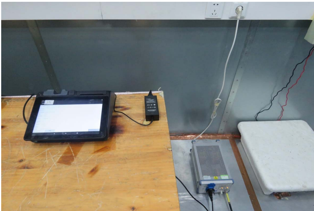
Picture 2 Conducted Emission Test Setup
