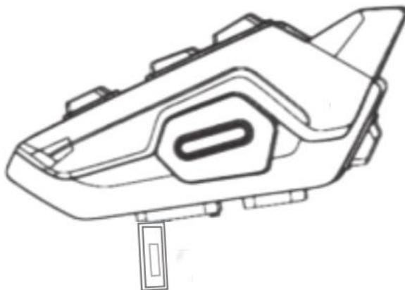
Open the plastic plug to expose the charging socket.
