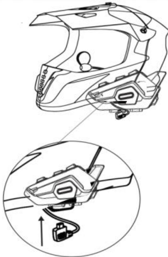
Connect the plug of the Microphone & Ear Speaker to the Microphone & Ear Speaker Socket of the headset.
