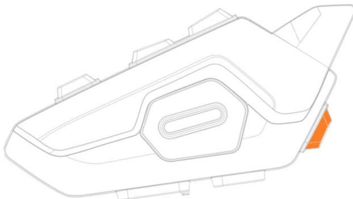
**Power on:** Press and hold **【on/off】** for 2 seconds, hear the power on tone, Blue light on for 1 second, then turn to every 2 seconds fast flashing blue light twice.
