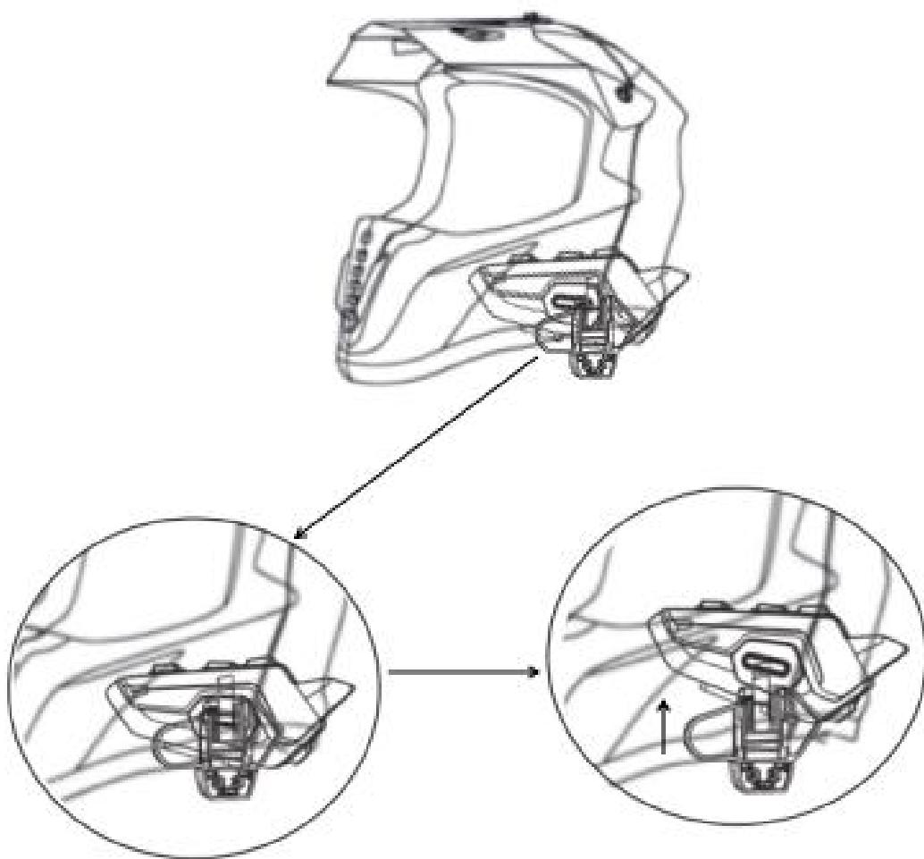
Press the plastic protruding stick of the clamp inwards while pressing the protruding stick of the clamp, take out the headset.
