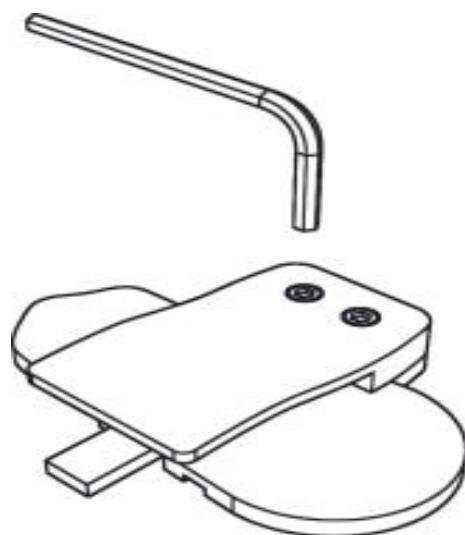
use the Allen key to loosen the bracket of the clamp.
