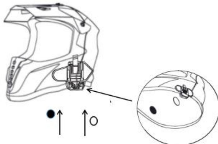
attach the circle magic sticker to the inner right & left sides of your helmet (it needs to be installed close to the ear position of the helmet to achieve best volume sound effect.)
