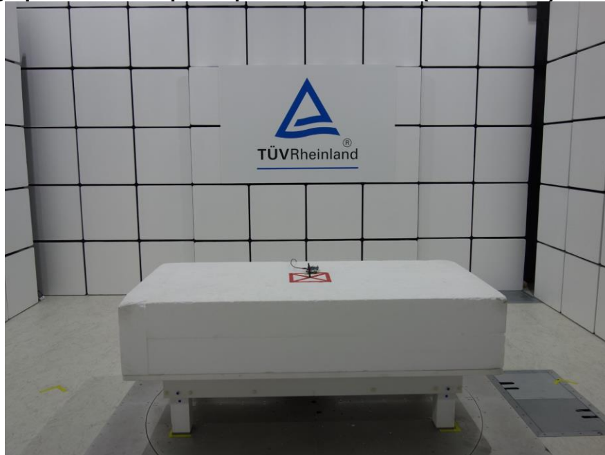
Photograph 2: Test Setup for Spurious Emissions (Front View 2)
