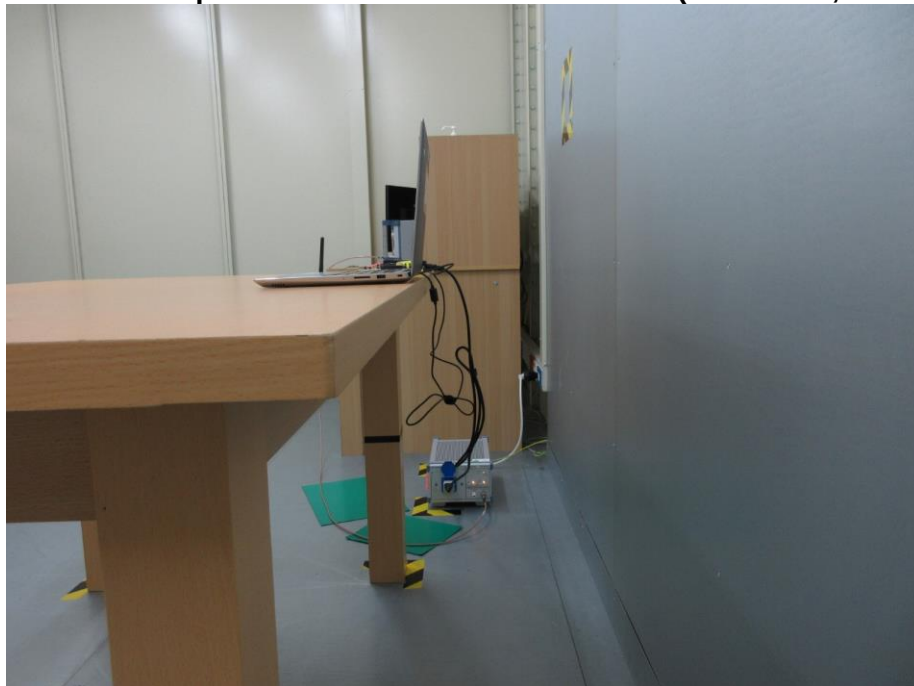
Photograph 22: Test Setup for Mains Conducted Emissions (Back View, MSK32WT-M13)
