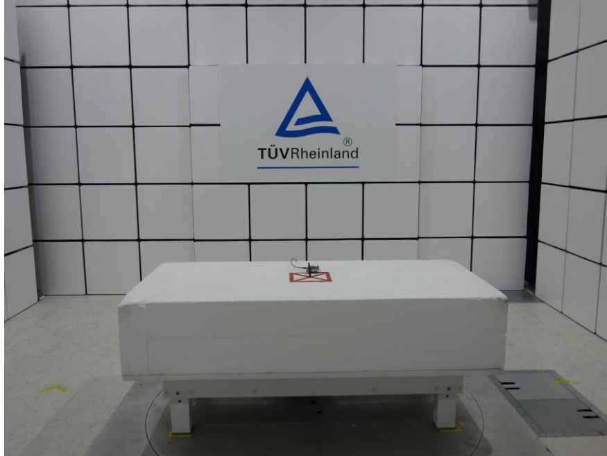
Photograph 9: Test Setup for Spurious Emissions (Front View 1, MSK32WT-M13, BLE)
