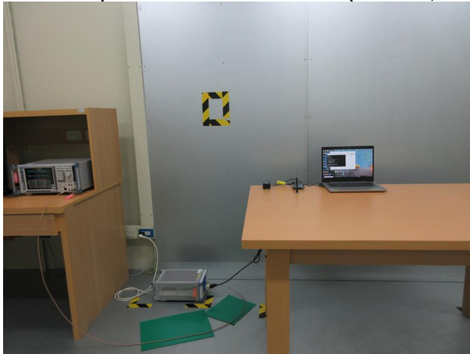
Photograph 22: Test Setup for Mains Conducted Emissions (Back View, MSK32WT-M13)
