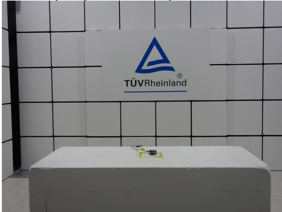
Photograph 1: Test Setup for Spurious Emissions (Front View 1, MSK32WT-M10)
