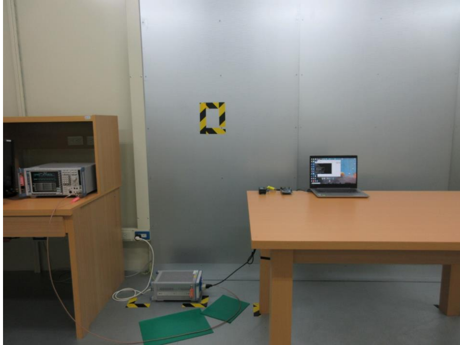
Photograph 7: Test Setup for Mains Conducted Emissions (Front View, MSK32WT-M10)
