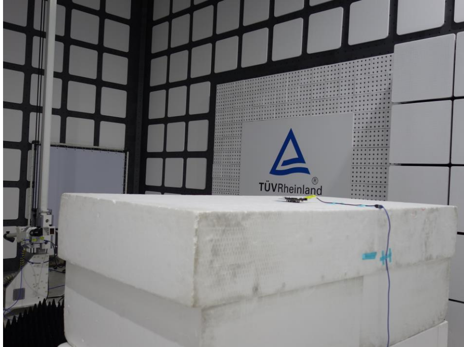
Photograph 3: Test Setup for Spurious Emissions (Back View 1, MSK32WT-M10)
