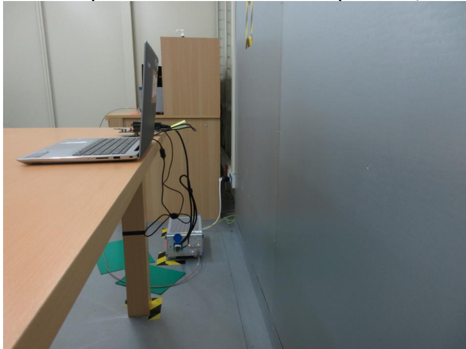
Photograph 8: Test Setup for Mains Conducted Emissions (Back View, MSK32WT-M10)
