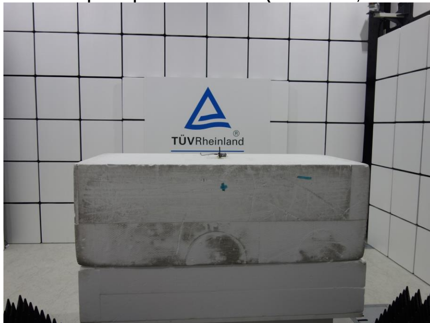
Photograph 10: Test Setup for Spurious Emissions (Front View 2, MSK32WT-M13, BLE)
