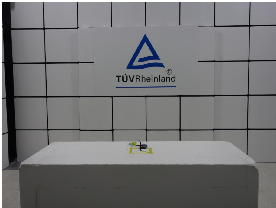
Photograph 16: Test Setup for Spurious Emissions (Front View 2, MSK32WT-M13, ZIGBEE)
