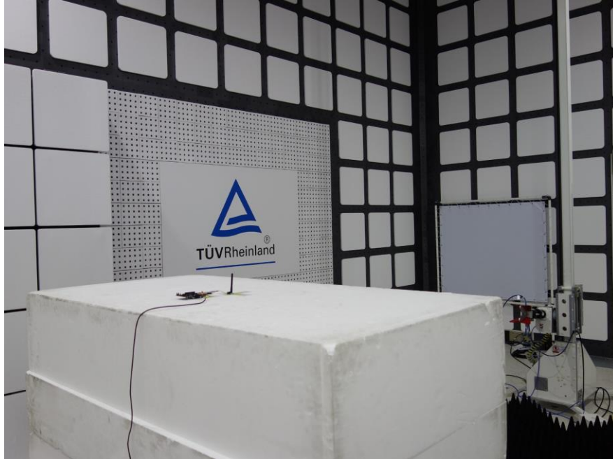
Photograph 13: Test Setup for Spurious Emissions (Back View 3, MSK32WT-M13, BLE)
