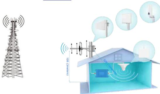
1. Connect the 50ft Coaxial Cable to the Outdoor Yagi/PLA/Panel/Tube Antenna
