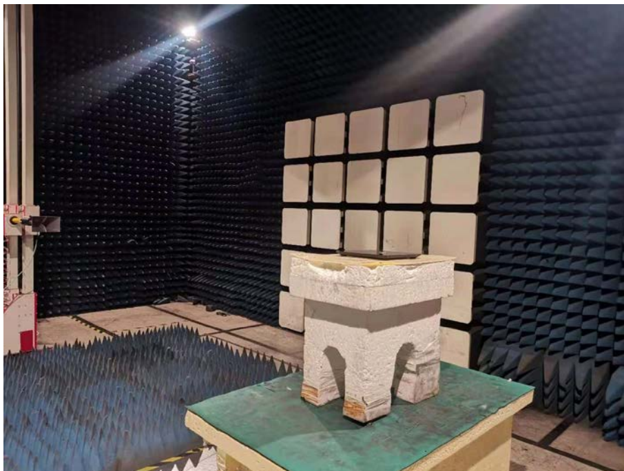
Spurious Emission Test Setup (Above 1GHz)
