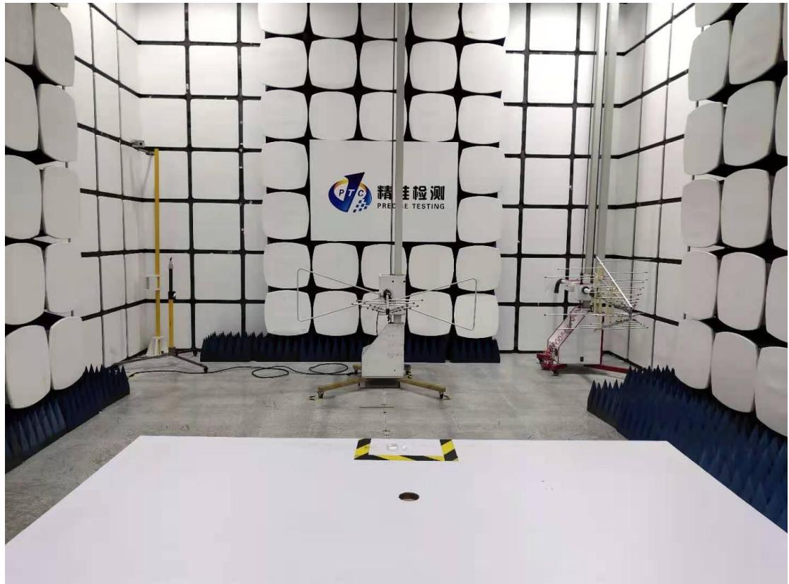
Test frequency from 1GHz-18GHz
