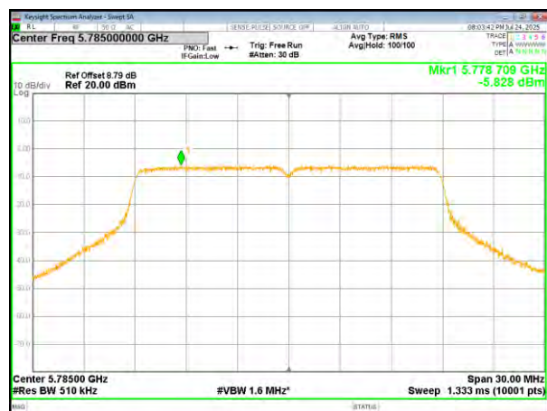
(802.11ac20) PSD plot on channel 165
