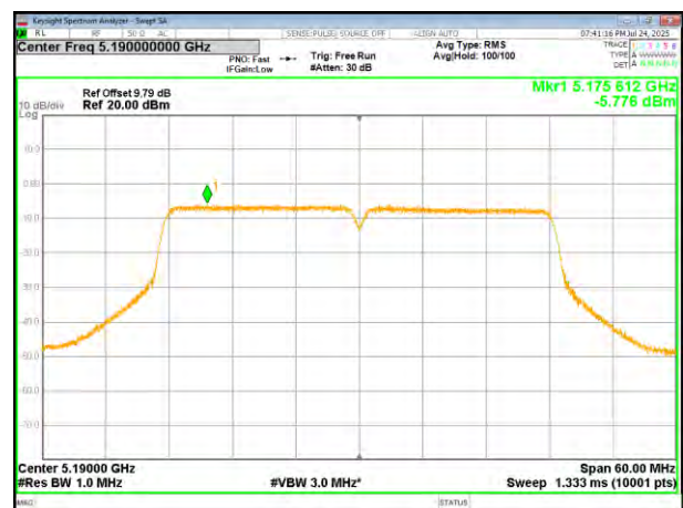
(802.11ac40) PSD plot on channel 38
