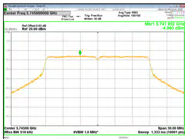
(802.11ac20) PSD plot on channel 149
