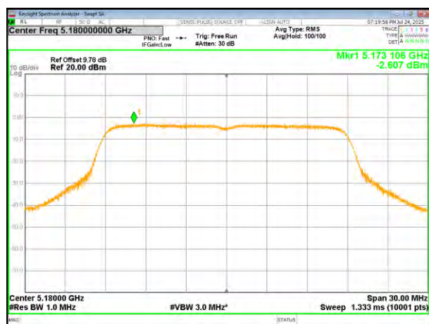
(802.11n20) PSD plot on channel 40
