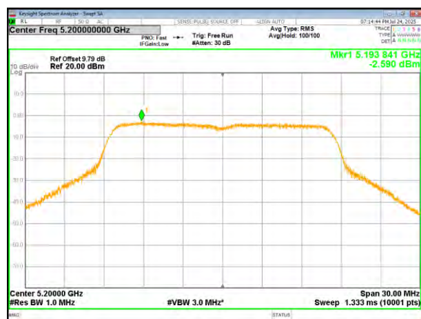
(802.11a) PSD plot on channel 48
