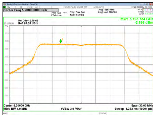
(802.11ac20) PSD plot on channel 48
