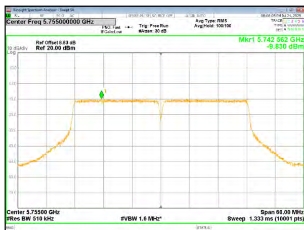
(802.11n40) PSD plot on channel 151
