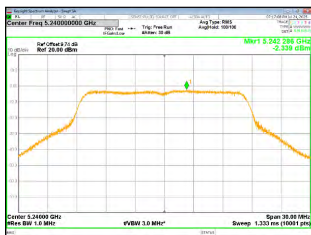
(802.11a) PSD plot on channel 48
