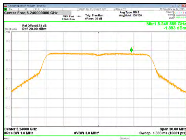
(802.11ac20) PSD plot on channel 48
