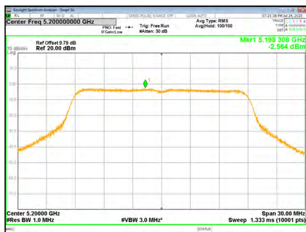
(802.11n20) PSD plot on channel 48
