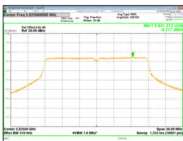
(802.11n20) PSD plot on channel 165
