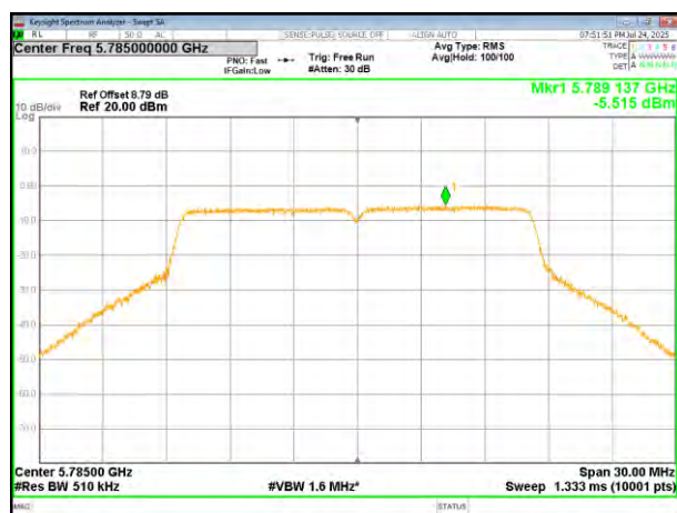
(802.11a) PSD plot on channel 165
