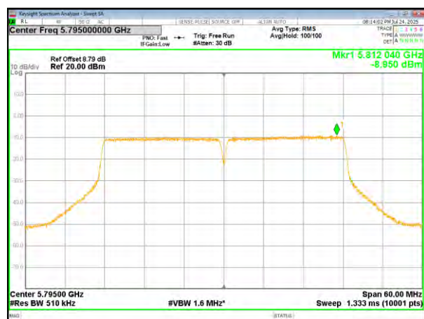
(802.11ac40) PSD plot on channel 159
