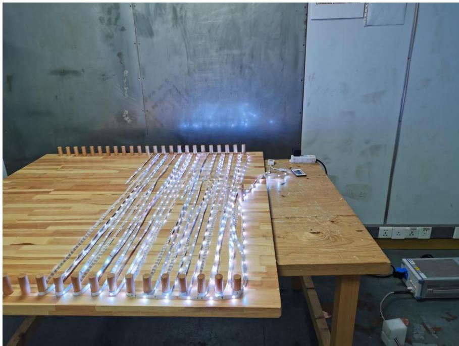
2. Photo of Radiated Emission Measurement (Below 1G)
