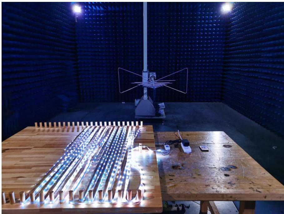
3. Photo of Radiated Emission Measurement (Above 1G)
