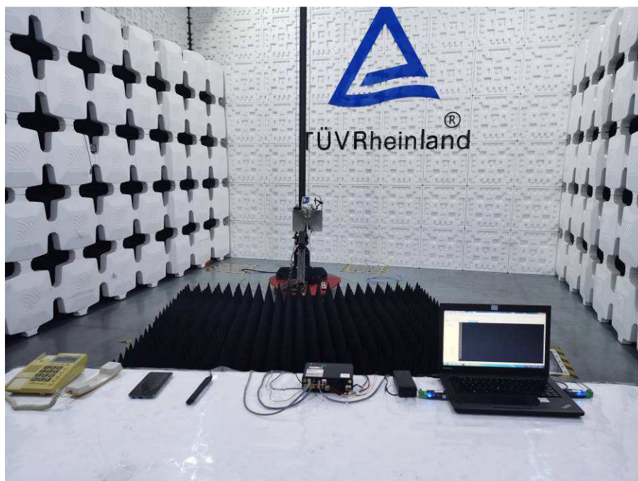
Photograph 3: Set-up photo for Radiated Emission, Above 1GHz
