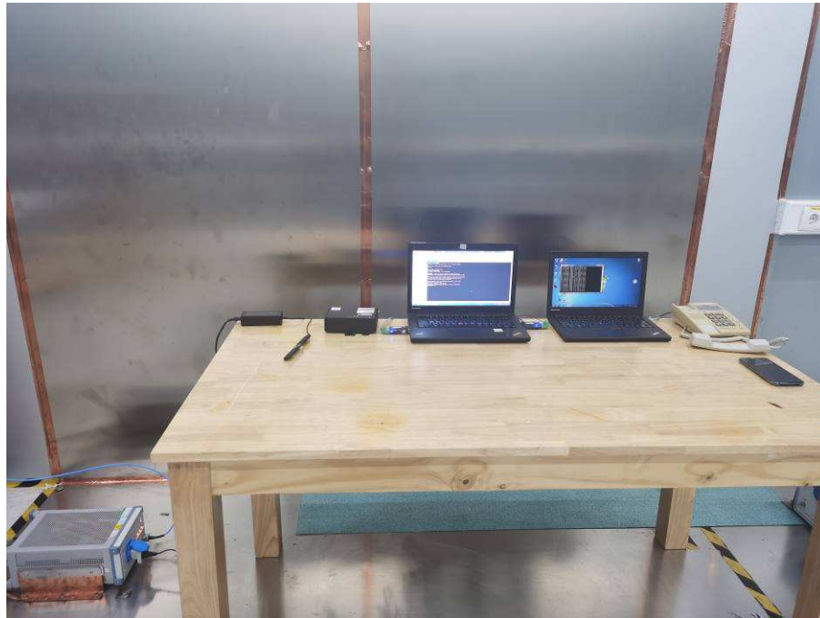
Photograph 1: Set-up for Conducted Emission on AC Mains
