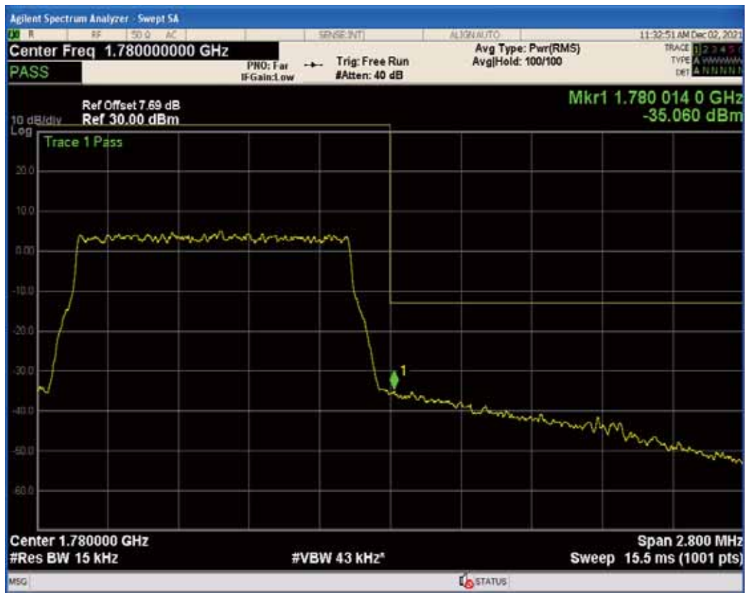
Band66 QAM16 BW=20MHz Channel=132072 RB Size=1 Position=#0
