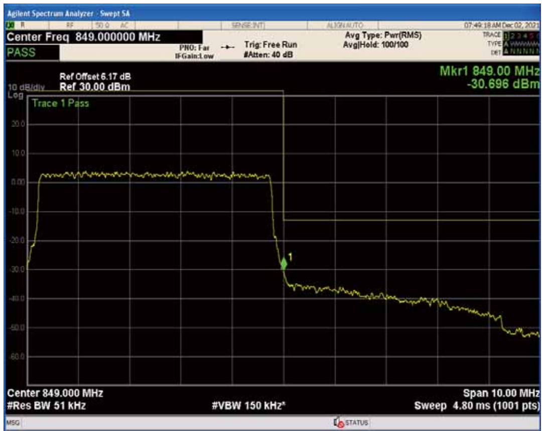
Band5 QPSK BW=5MHz Channel=20625 RB Size=1 Position=#Max
