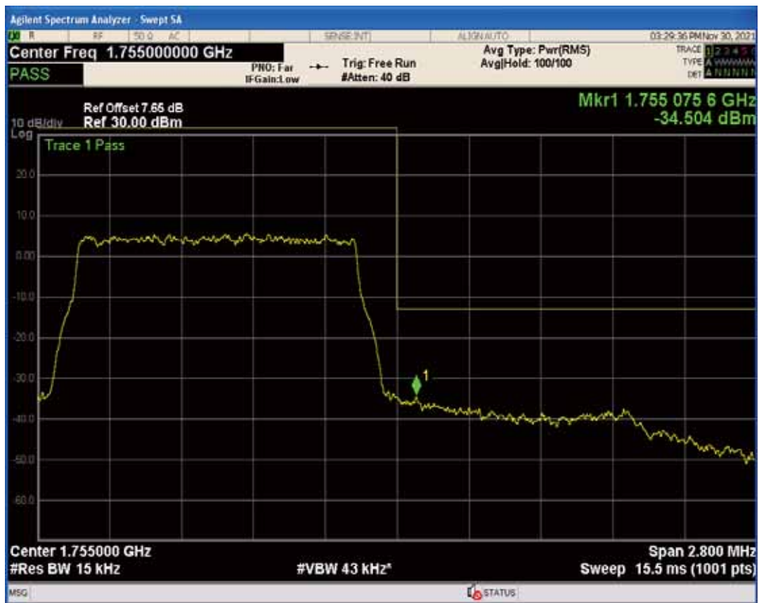
Band4 QPSK BW=1.4MHz Channel=20393 RB Size=1 Position=#Max
