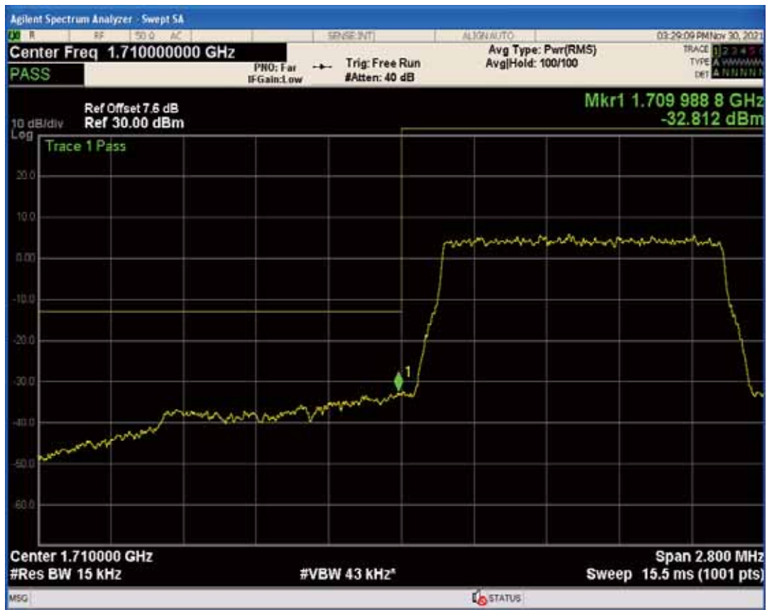
Band4 QPSK BW=1.4MHz Channel=20393 RB Size=6 Position=#0
