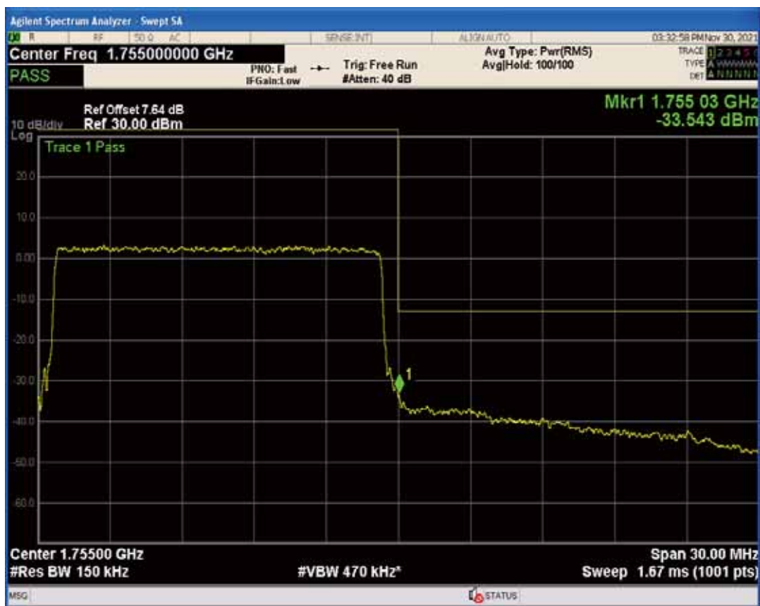
Band4 QAM16 BW=15MHz Channel=20325 RB Size=1 Position=#Max
