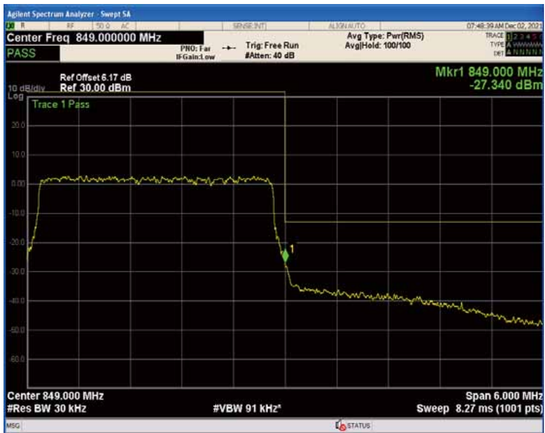
Band5 QAM16 BW=3MHz Channel=20635 RB Size=1 Position=#Max
