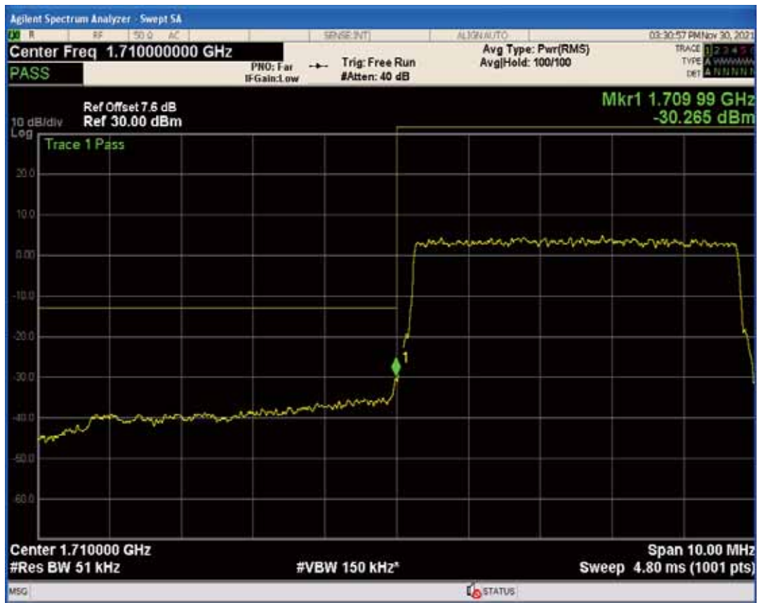
Band4 QPSK BW=5MHz Channel=20375 RB Size=1 Position=#0
