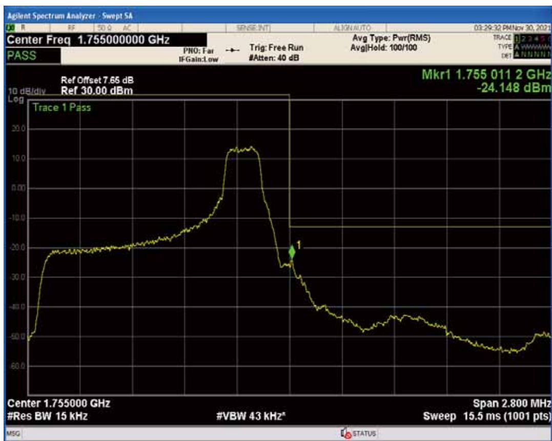
Band4 QPSK BW=20MHz Channel=20050 RB Size=1 Position=#0
