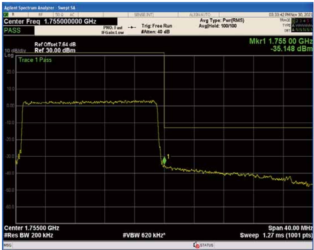
Band4 QAM16 BW=3MHz Channel=19965 RB Size=1 Position=#0
