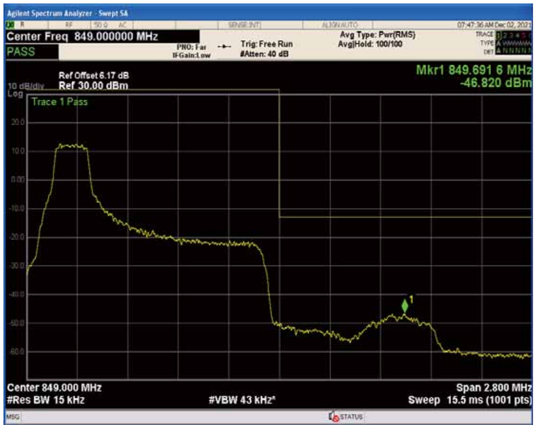
Band5 QAM16 BW=10MHz Channel=20600 RB Size=1 Position=#0
