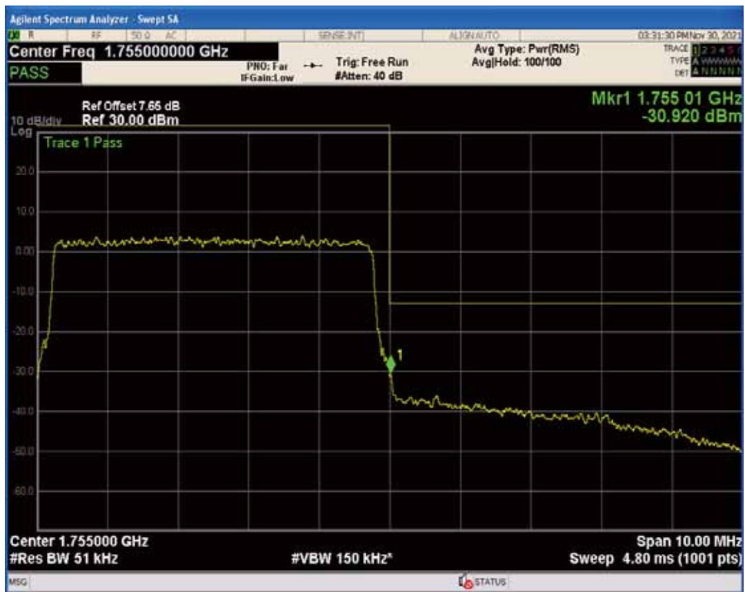
Band4 QPSK BW=1.4MHz Channel=19957 RB Size=1 Position=#0
