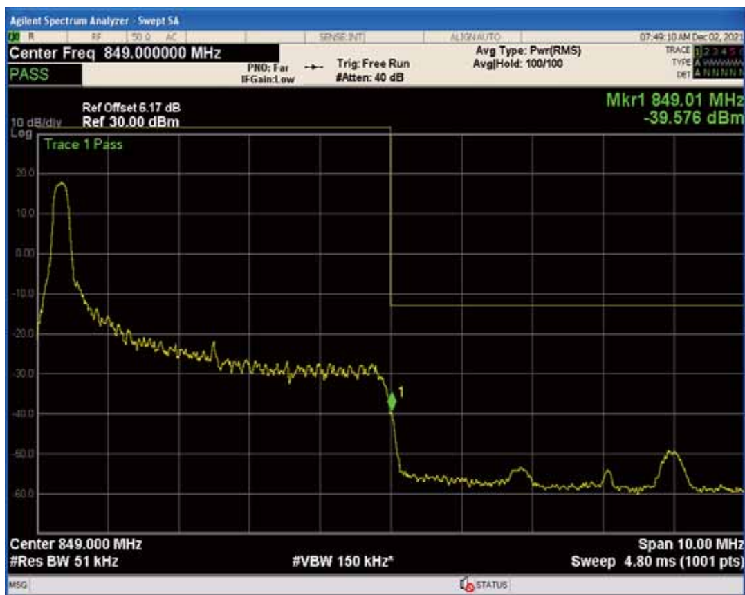
Band5 QPSK BW=5MHz Channel=20625 RB Size=25 Position=#0
