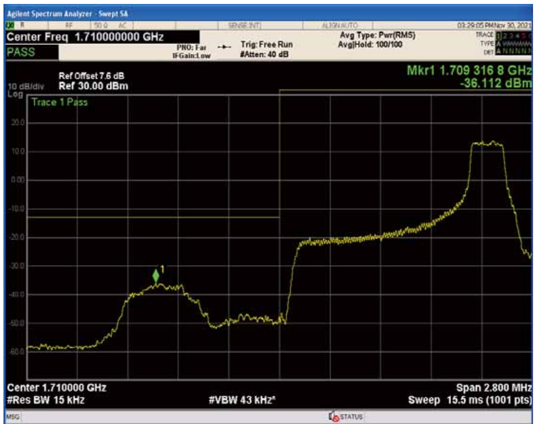
Band4 QAM16 BW=5MHz Channel=20375 RB Size=1 Position=#Max
