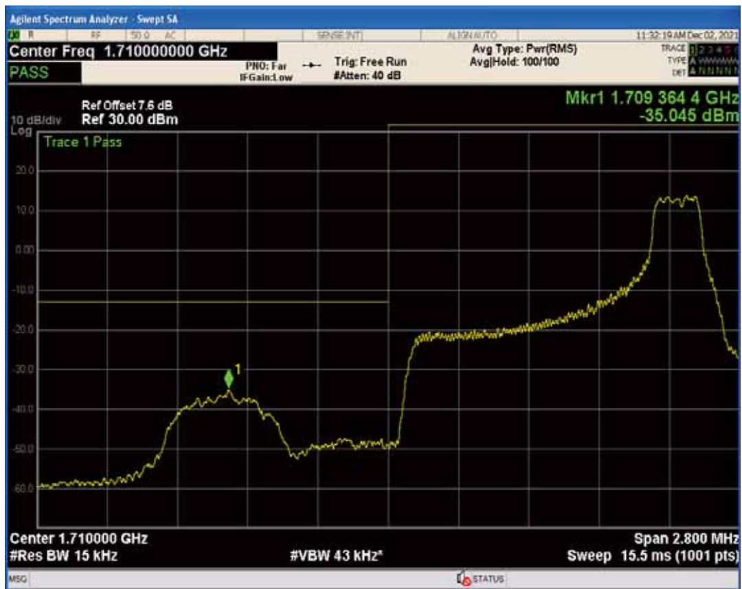
Band66 QAM16 BW=1.4MHz Channel=131979 RB Size=1 Position=#0
