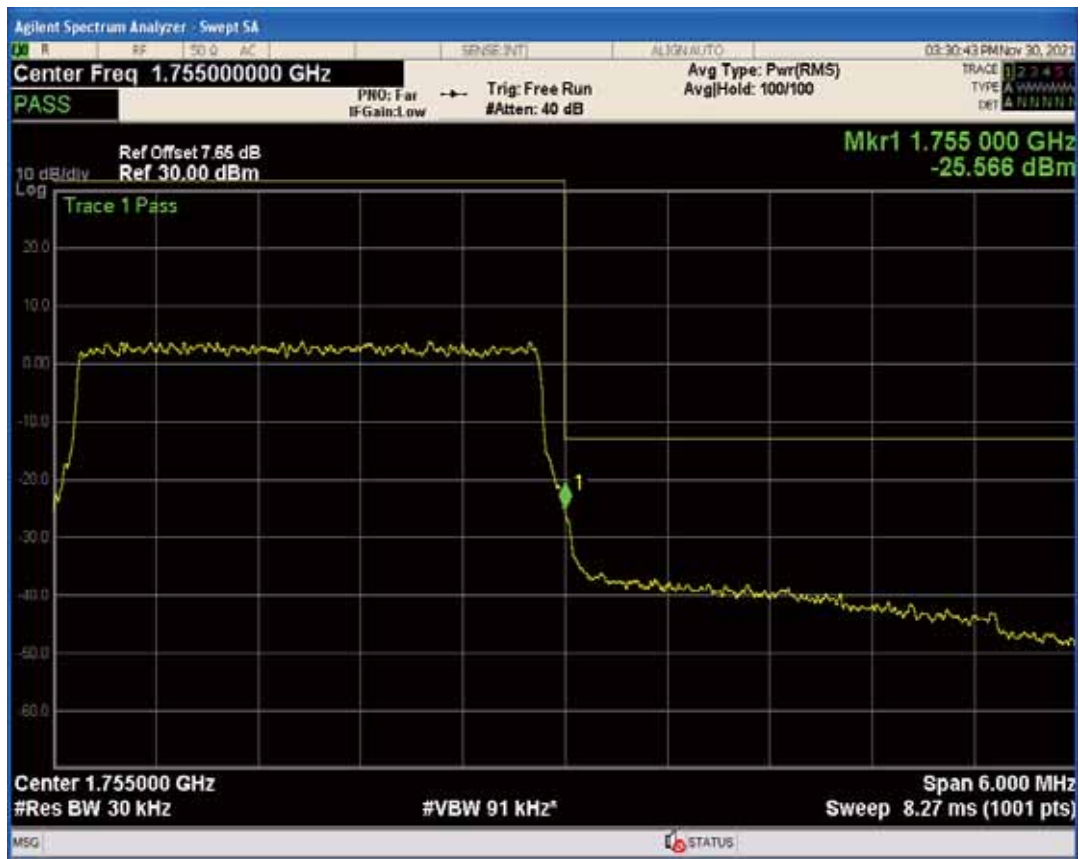
Band4 QAM16 BW=5MHz Channel=19975 RB Size=1 Position=#0
