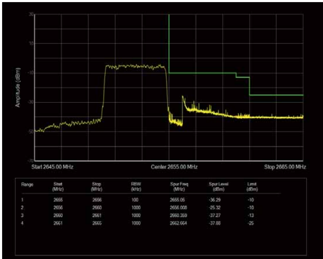
Band41 QPSK BW=5MHz Channel=40065 RB Size=1 Position=#0
