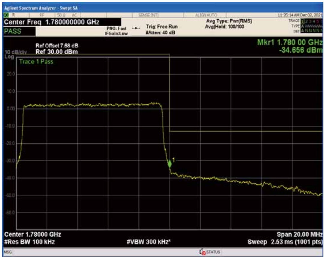
Band66 QAM16 BW=15MHz Channel=132047 RB Size=1 Position=#Max
