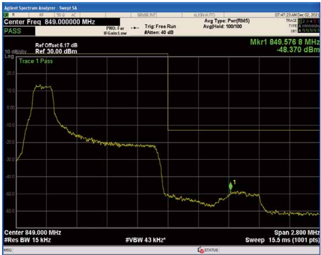
Band5 QPSK BW=1.4MHz Channel=20407 RB Size=6 Position=#0
