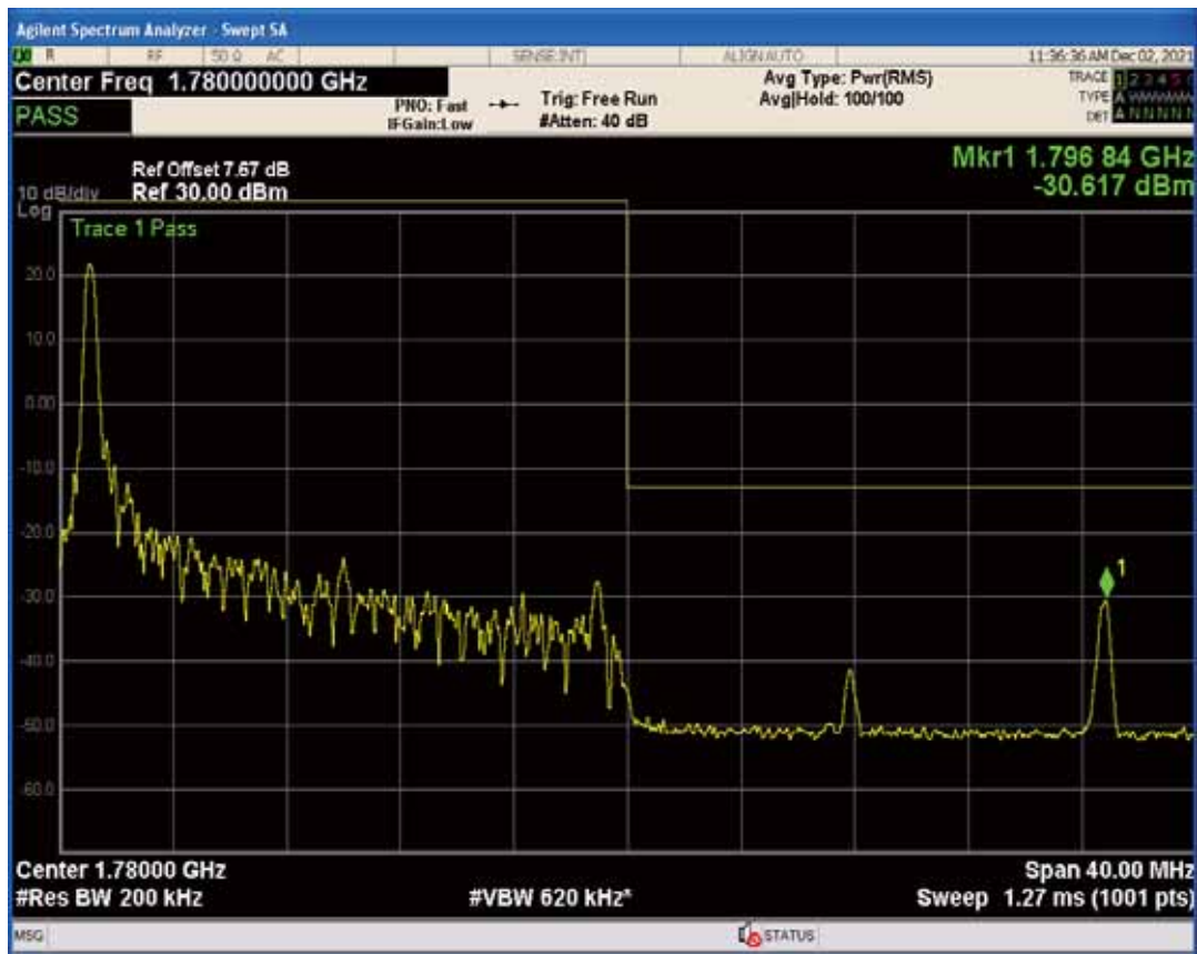
Band66 QAM16 BW=20MHz Channel=132072 RB Size=100 Position=#0
