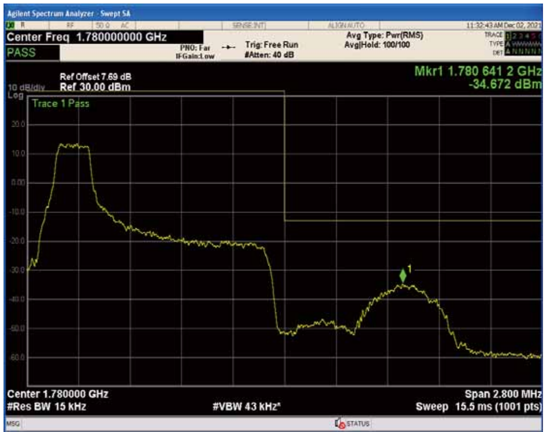
Band66 QAM16 BW=10MHz Channel=132022 RB Size=1 Position=#0
