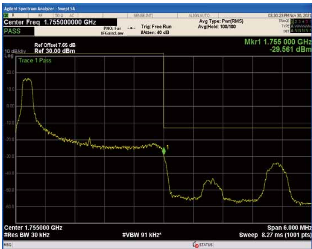
Band4 QPSK BW=3MHz Channel=20385 RB Size=1 Position=#Max
