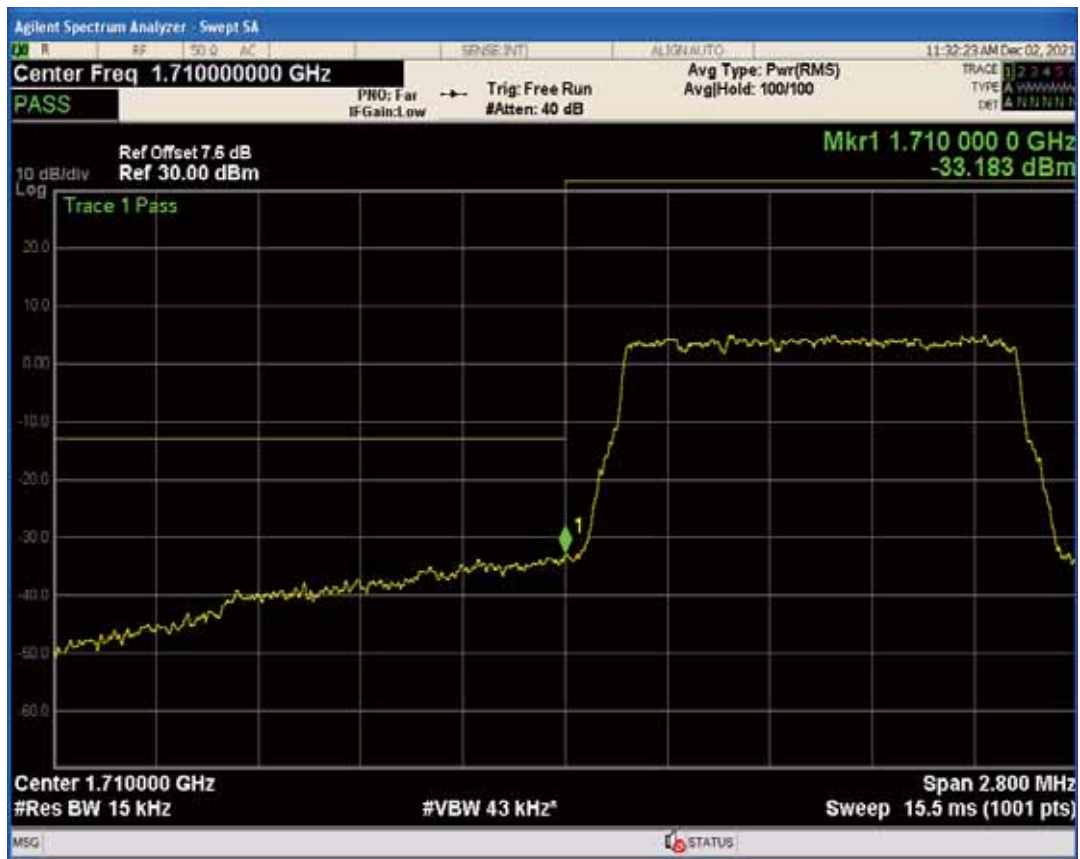
Band66 QAM16 BW=1.4MHz Channel=131979 RB Size=1 Position=#Max
