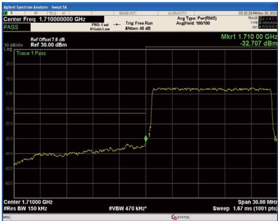
Band4 QPSK BW=3MHz Channel=19965 RB Size=1 Position=#Max
