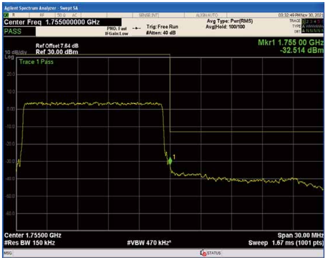
Band4 QPSK BW=20MHz Channel=20050 RB Size=1 Position=#Max
