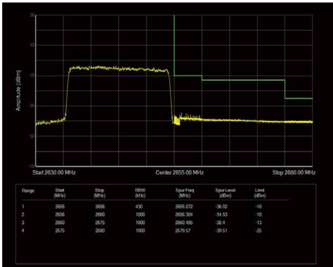
Band41 QPSK BW=20MHz Channel=40140 RB Size=100 Position=#0
