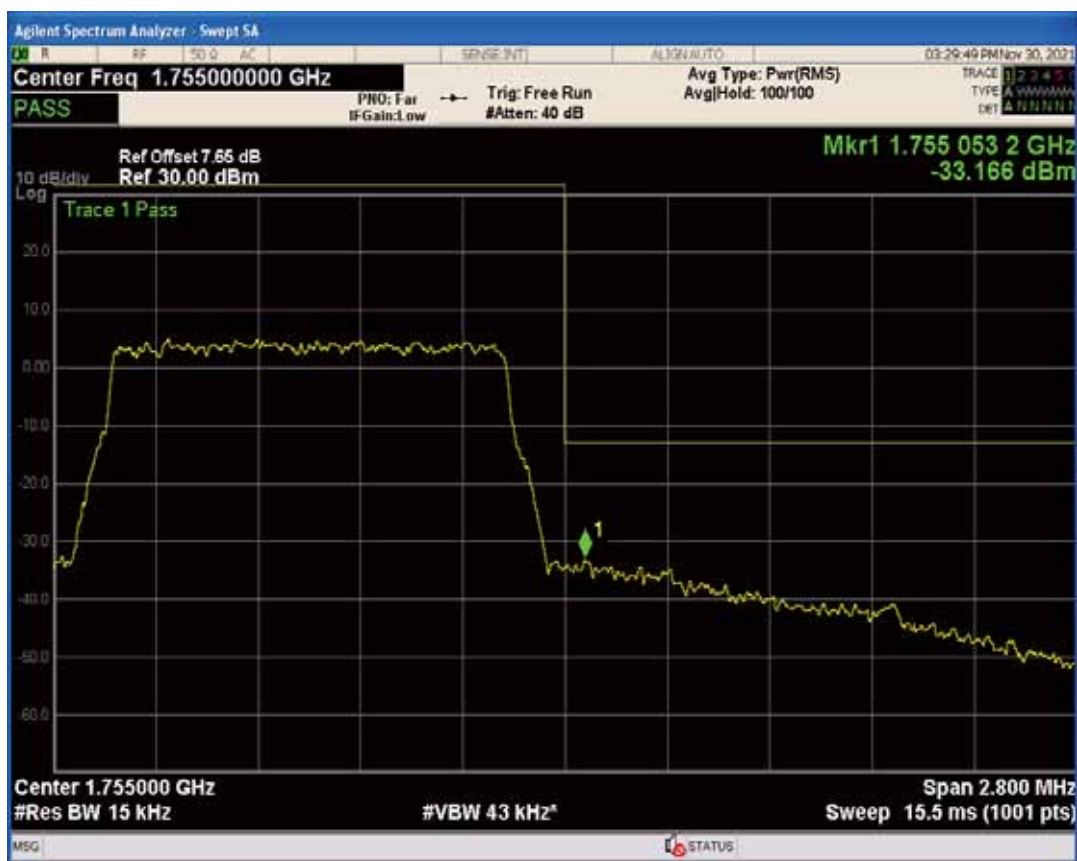
Band4 QAM16 BW=10MHz Channel=20000 RB Size=1 Position=#0
