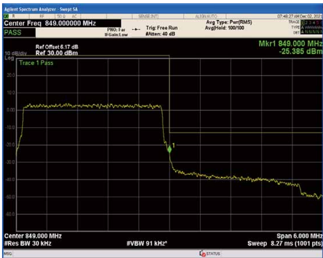
Band5 QPSK BW=3MHz Channel=20635 RB Size=1 Position=#Max
