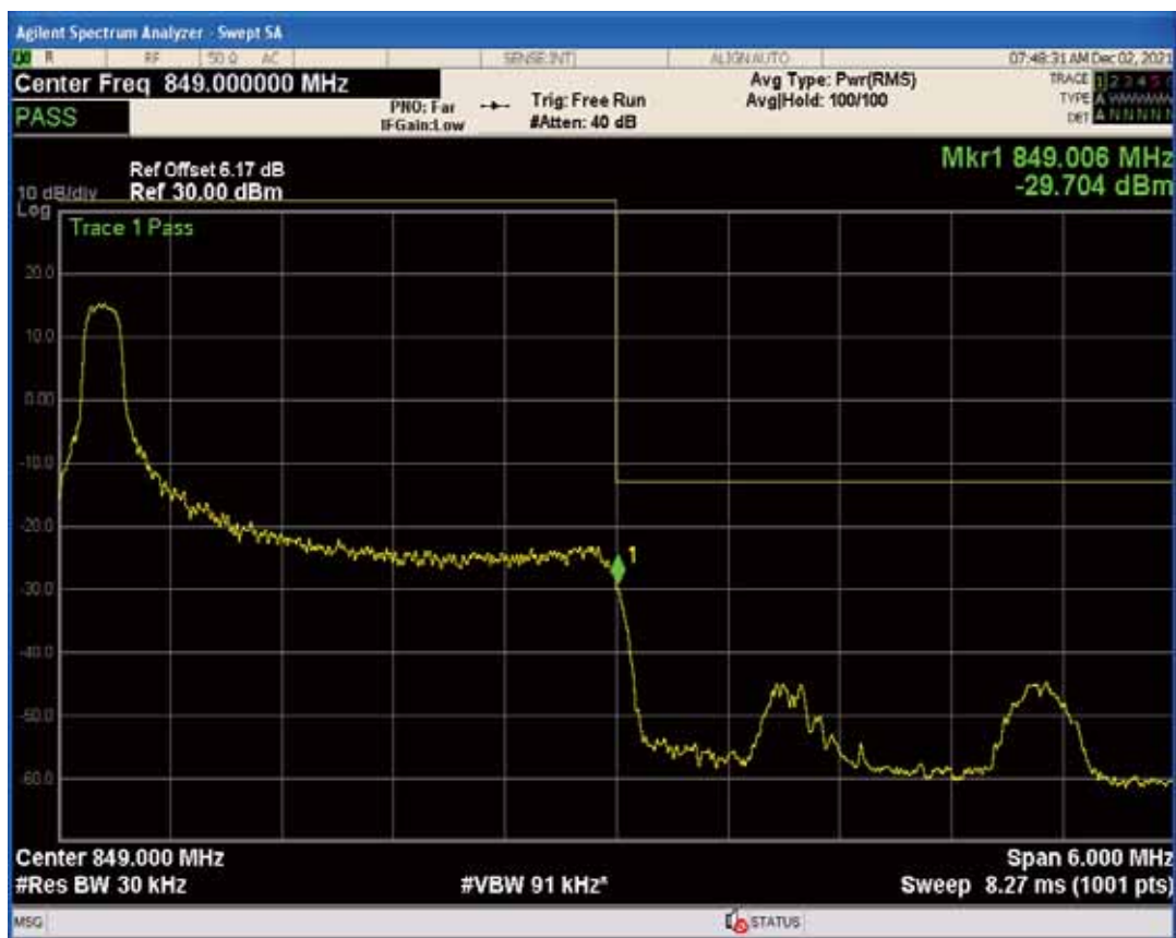
Band5 QAM16 BW=3MHz Channel=20415 RB Size=15 Position=#0
