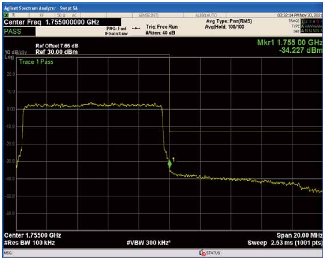
Band4 QAM16 BW=15MHz Channel=20025 RB Size=1 Position=#0
