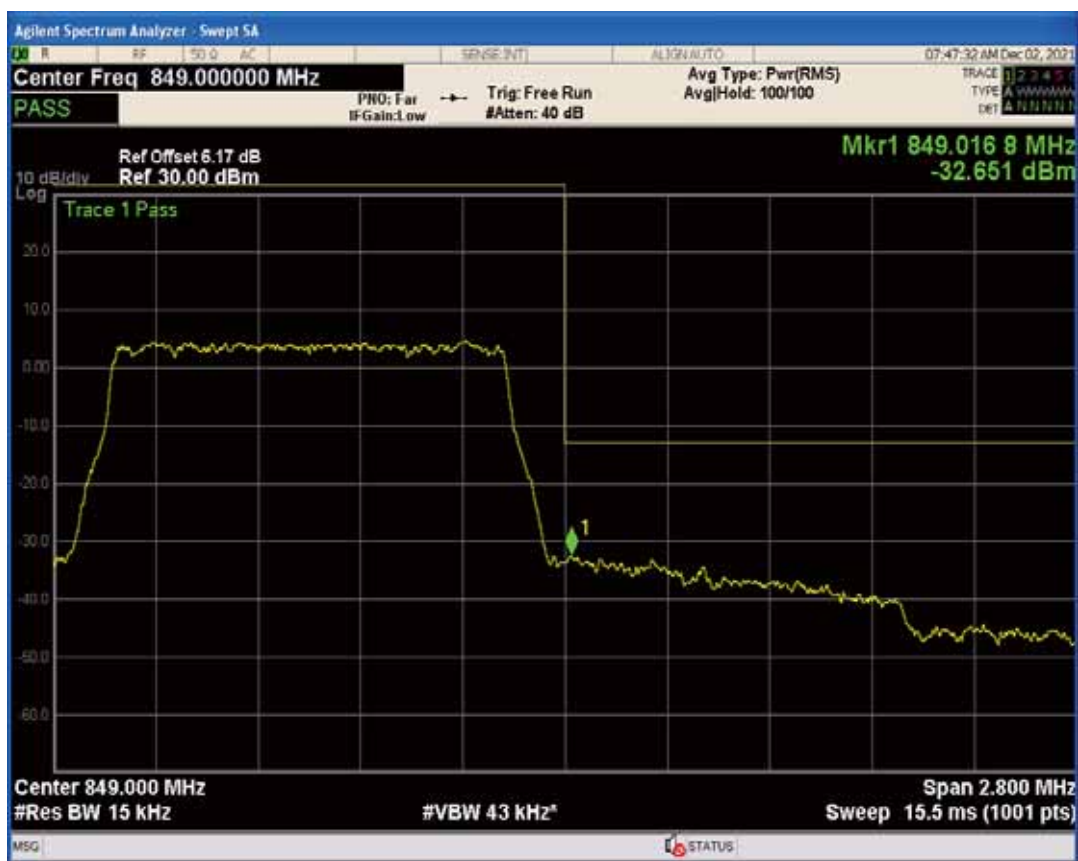
Band5 QPSK BW=5MHz Channel=20425 RB Size=25 Position=#0
