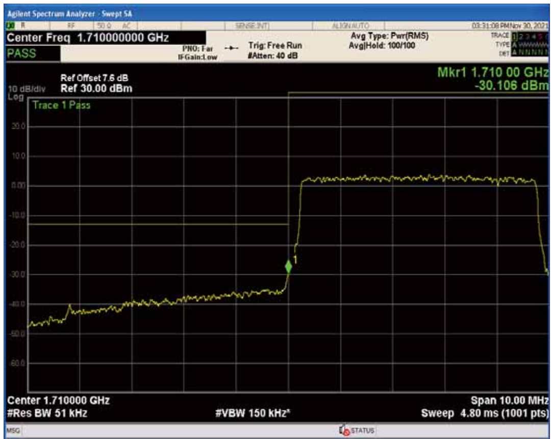
Band4 QAM16 BW=5MHz Channel=20375 RB Size=1 Position=#0
