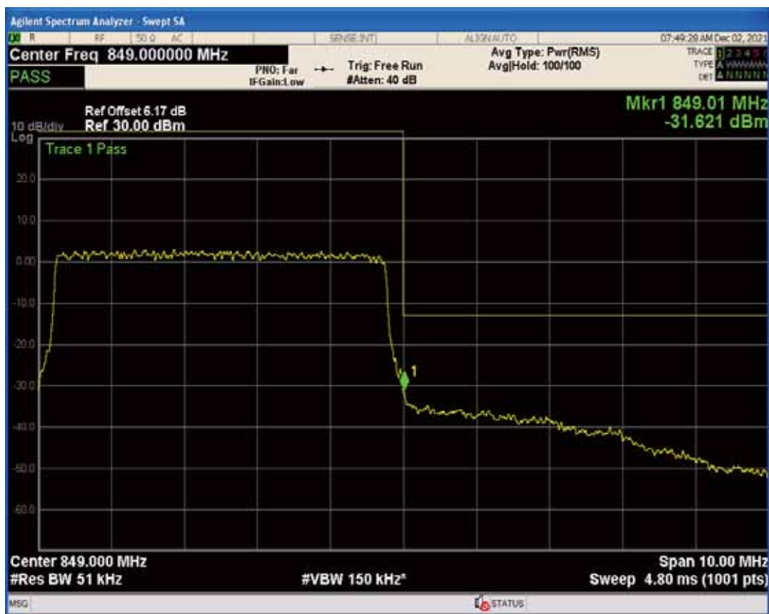
Band5 QAM16 BW=5MHz Channel=20625 RB Size=1 Position=#0
