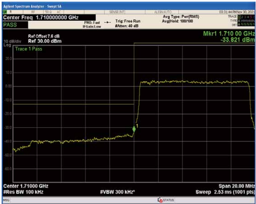
Band4 QPSK BW=10MHz Channel=20000 RB Size=1 Position=#Max
