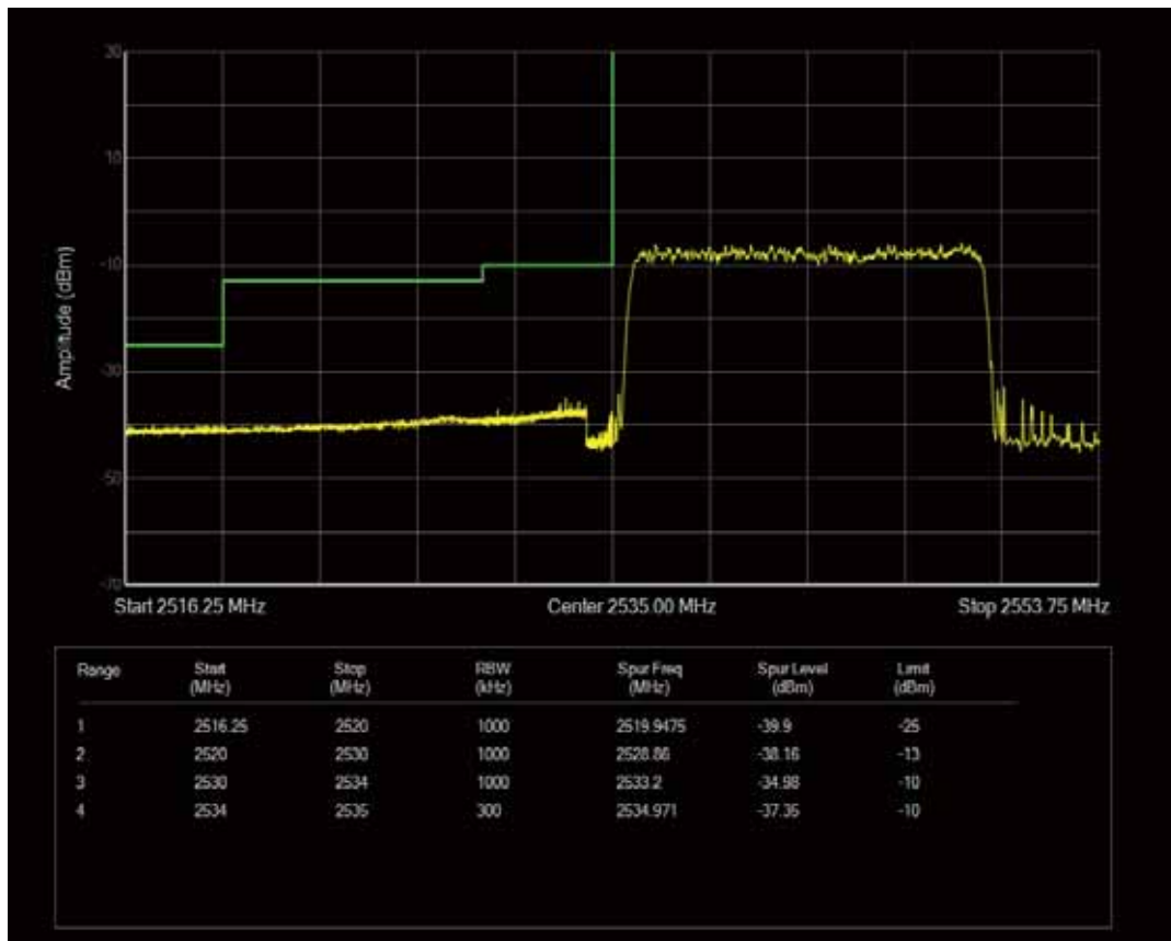
Band41 QAM16 BW=10MHz Channel=40090 RB Size=1 Position=#Max
