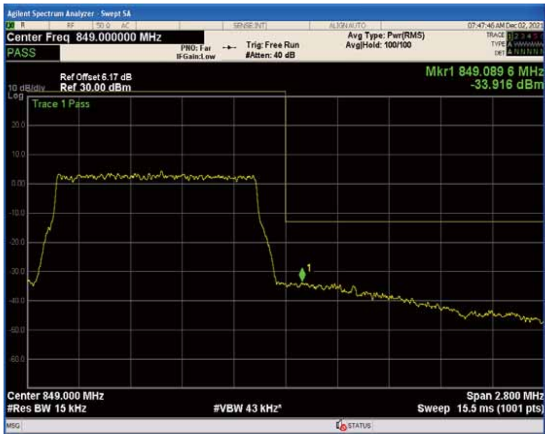
Band5 QAM16 BW=10MHz Channel=20450 RB Size=1 Position=#0
