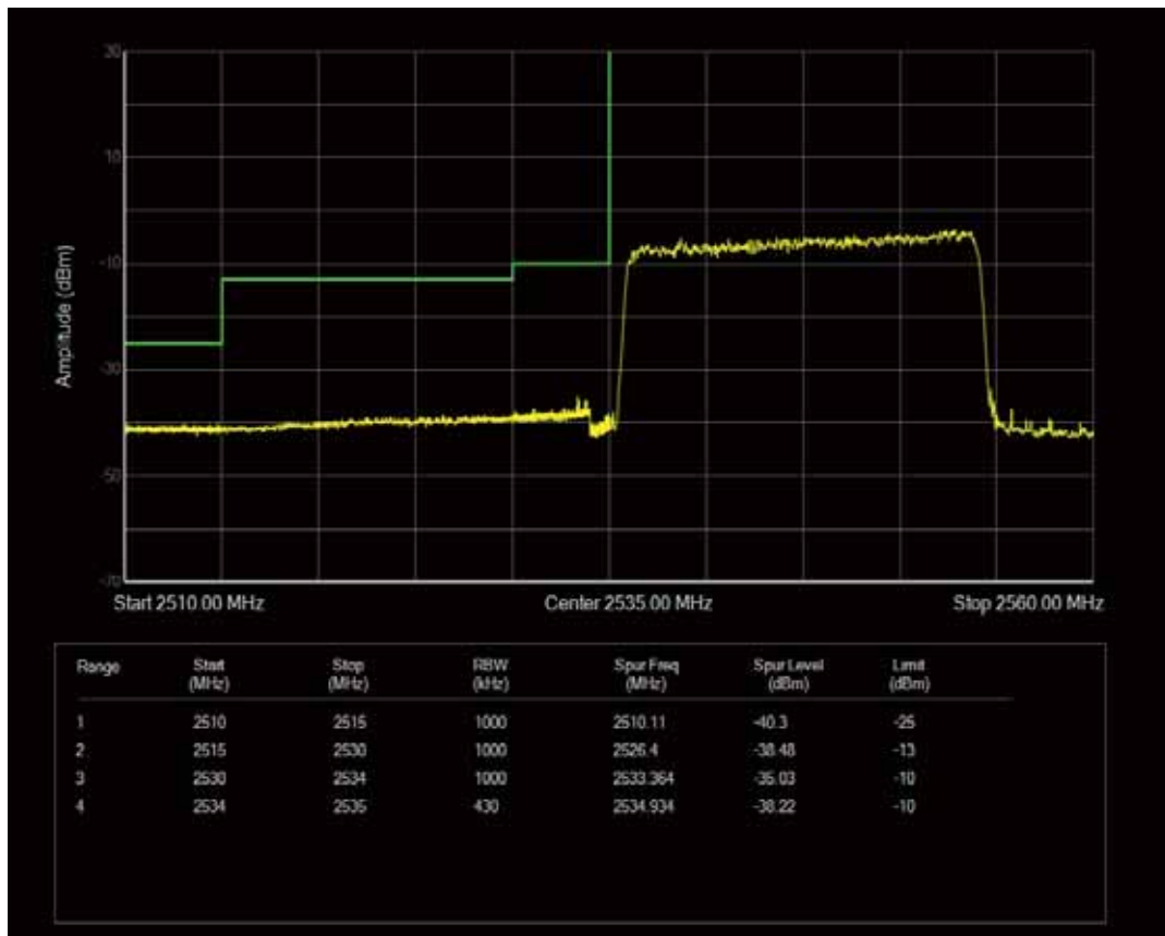
Band41 QPSK BW=20MHz Channel=41140 RB Size=1 Position=#0
