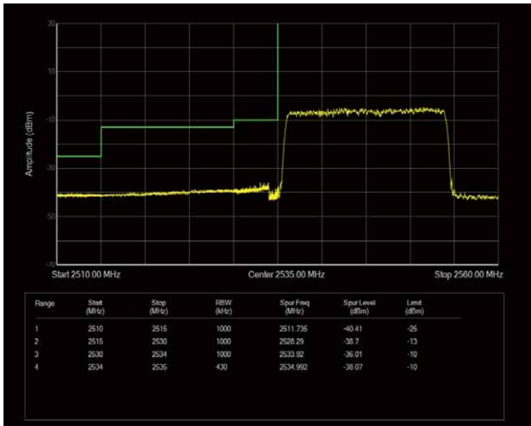
Band41 QAM16 BW=20MHz Channel=41140 RB Size=1 Position=#0
