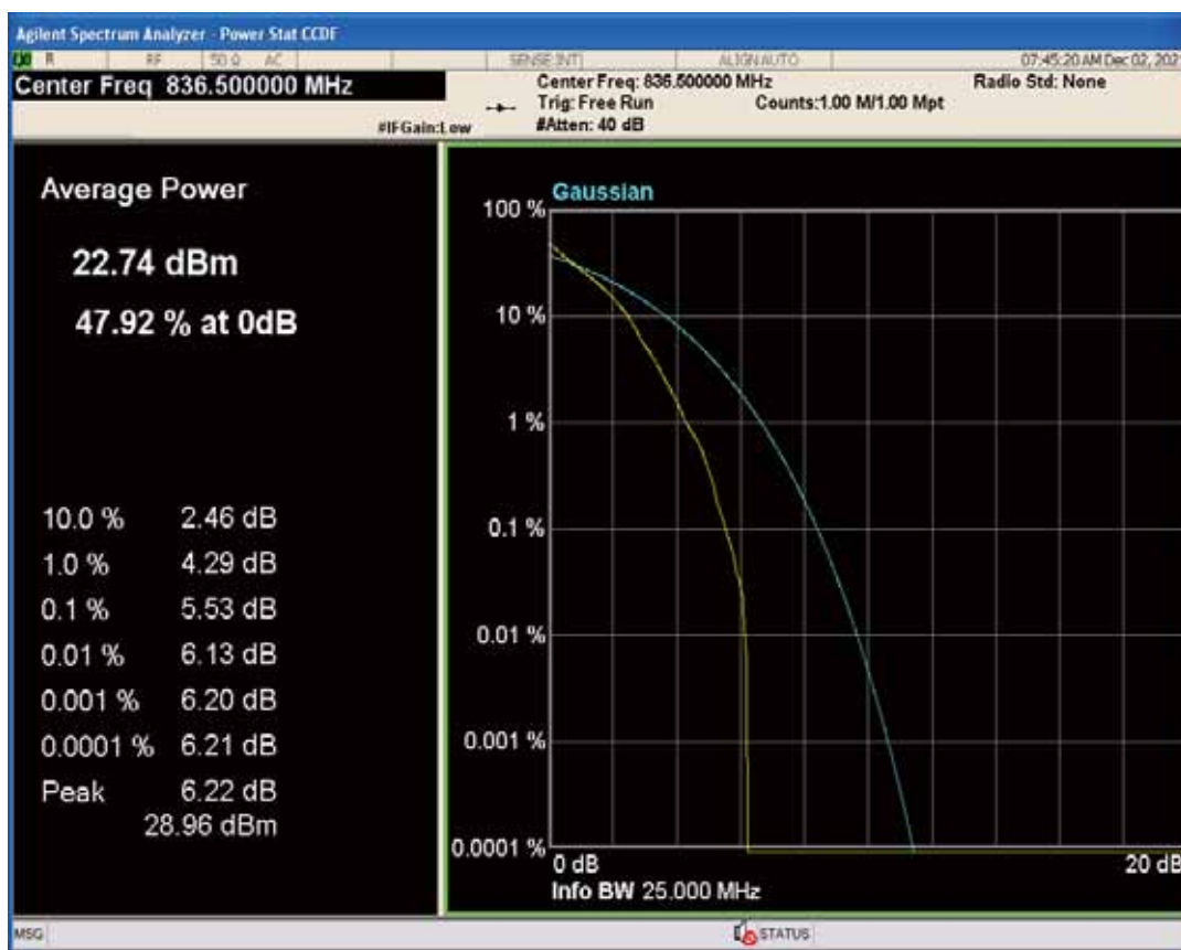
Band5 QAM16 BW=10MHz Channel=20525 RB Size=1 Position=#0
