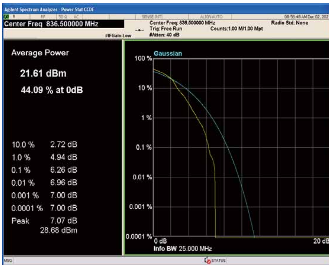
Band26b QAM16 BW=3MHz Channel=26915 RB Size=1 Position=#0
