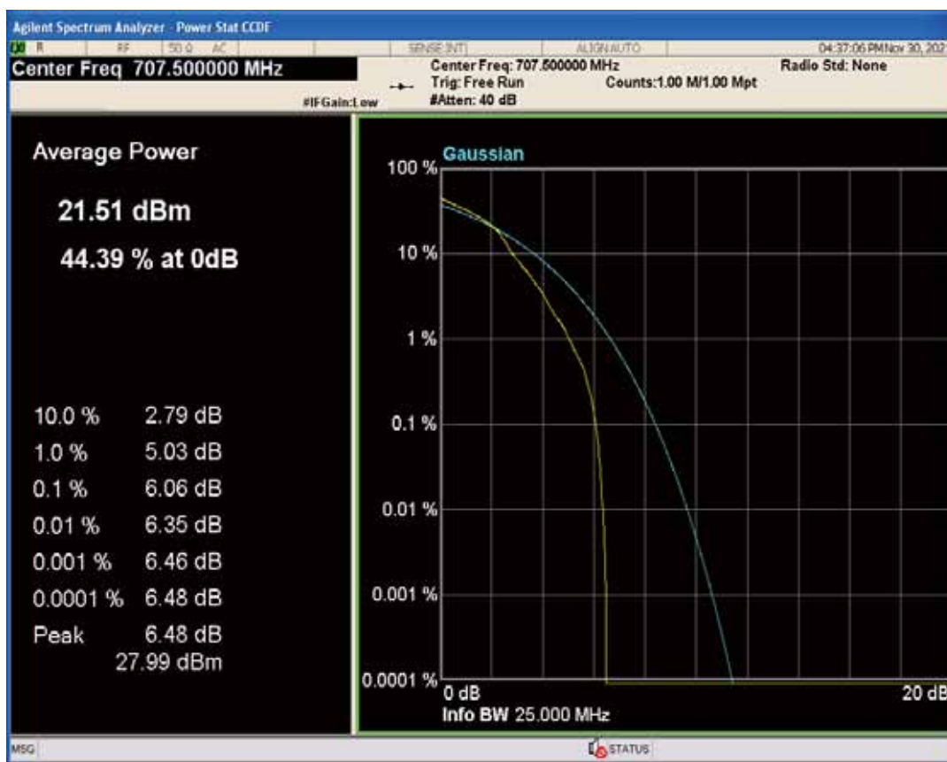
Band12 QAM16 BW=1.4MHz Channel=23095 RB Size=1 Position=#0
