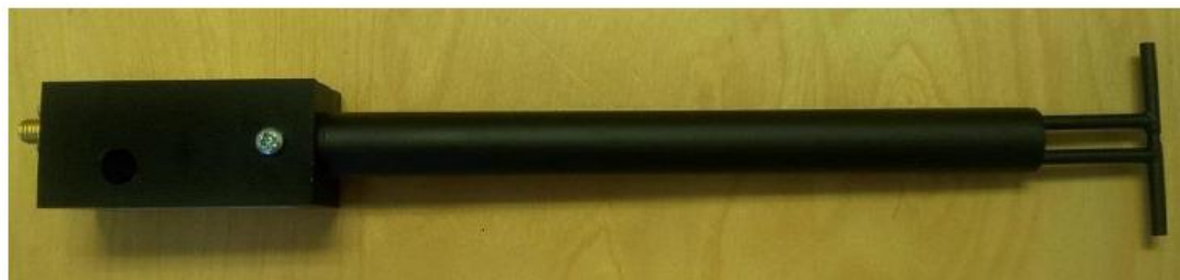
Figure 1 – MVG COMOSAR Validation Dipole
