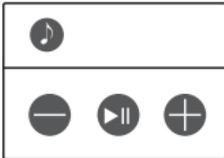
Long press Vol-
